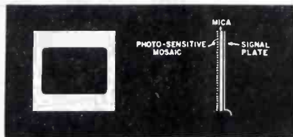
Fig. 2. Signal plate used in iconoscope, consisting of sheet of mica, the front of which is coated with a photo-sensitive material.
