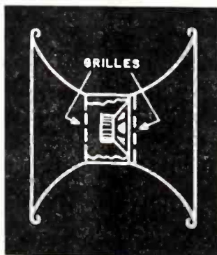
Fig. 8. One type of bi-directional cone baffle utilizing both back and front radiation.
