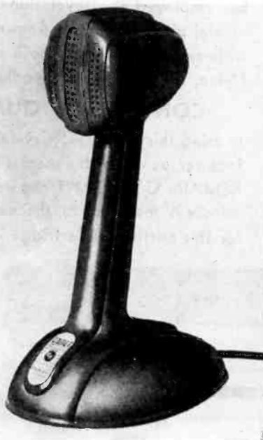
Fig. 9. Combination crystal microphone and desk stand. Frequency response is 70 to 7,000 cps. Voltage developed by normal speech is .0394 volt.
