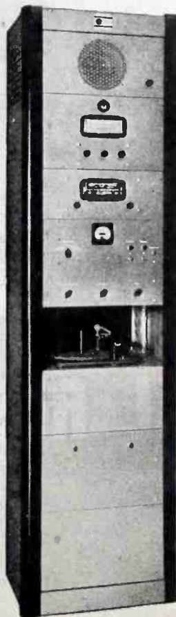
Fig. 2. A typical control rack used in war plant sound systems. Provided are a monitor speaker, a-m/f-m tuners, output level meter and switch panel, automatic record changer, and power amplifiers.
