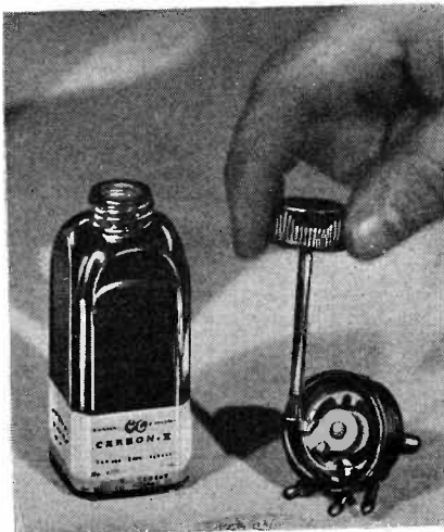
Fig. 1. "Carbon-X," a special liquid for "touching up" the resistance elements of moving carbon-type volume or tone controls, at worn, noisy spots.
