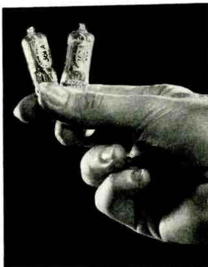
Midget type tubes have been designed especially for hearing aid devices.
