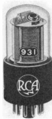
Figs. 1 and 1A. The RCA 931 is a multiplier type phototube that consists of an anode and a 9-stage electrically focused amplifier all housed in a 3 11/16 inch glass envelope.
