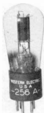
The Westinghouse Type 256A is a three-element, argon filled thyatron with an indirectly heated cathode and a five-pin base.
