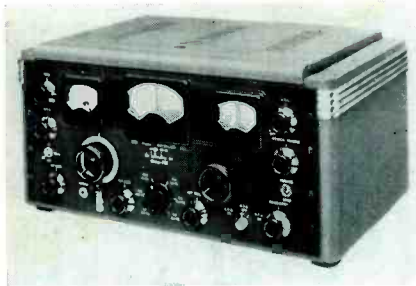
The intricate looking controls on the front panel of the SX28 provide those niceties of adjustment, such as calibrated band spread tuning and the like, which are expected from the communications receiver.
