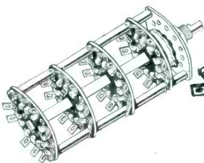
CENTRALAB SWITCHES WITH BAKELITE INSULATION
