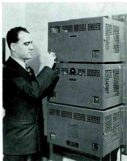
Fig. 5. Battery of high-power amplifiers develop electrical speech energy to direct the flow of traffic through the airlines terminal.
