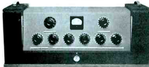
Fig. 4. (Above) In spite of the somewhat elaborate arrangement, the fair grounds installation is quite flexible and can be controlled from the remote console board shown in Fig. 3. This console permits control and mixing from any of four predetermined locations in the audience section.
