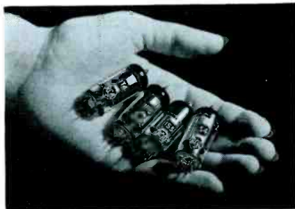
Fig. 1. The recently introduced seven-pin miniature tubes are quite well suited for use in hearing-aid amplifiers which employ an air-conduction earpiece. Sufficient gain and output can be obtained by employing a 1S5 followed by a 1T4.
