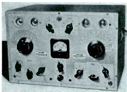
The Chanalyst was used to make the measurements indicated in the text and to obtain the readings shown on the opposite page. The method, in general, may be applied to other receivers using any similar signal tracer.
