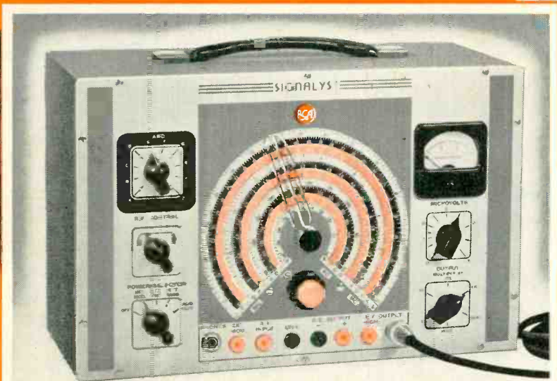
2 The RCA Signalyst... The Most Modern Signal Generator. Range—100Kc-120 Mc in fundamentals. Net Price $107.50
