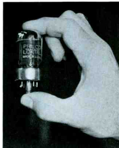
(Photo courtesy Philco) The relative size of the loktal tube can be determined by comparison with that of a man's hand.
