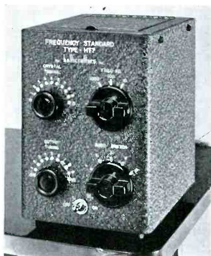
The 10-kc output of the Hallicrafters Model HT7 frequency standard has the advantage that precise checks of the receiver calibration in the broadcast band can be made by merely tuning the receiver dial through its range.
