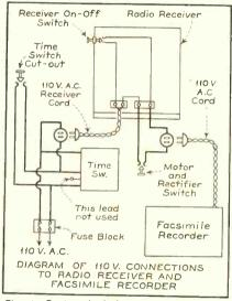
Fig. 4. During daylight and evening hours the time switch can be taken out of the circuit by operating the shunting switch to the on position. Application of power to the receiver is then controlled in normal manner with the regular off-on switch.
