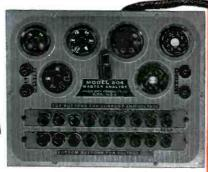
It seems RCP engineers have been working overtime. Laboratory 'info' says that the new Model 504 analyst will be ready March 1st. The Analyst an improved unique push button circuit selector—making possible grearer speed, safety and flexibility for analyzing symptoms at socket terminals in radio sets and P.A. installations.
