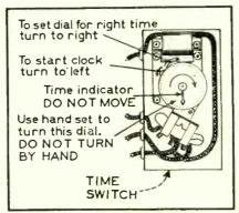
Fig. 5. There are twelve tapered pins provided with the time clock. Each pin is used in the proper hole to give one hour of light.
