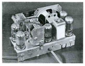
Loktal tubes enable this midget receiver to eliminate high-heat dissipating line-cord or ballast resistors and make it eligible for Underwriters' Laboratory approval.
