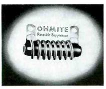
pressor is a non-inductive vitreous enamel resistor combined with a choke into one integral unit. For full details, write to Ohmite Mfg. Co., 4835 Flournoy St., Chicago. -- SERVICE.
