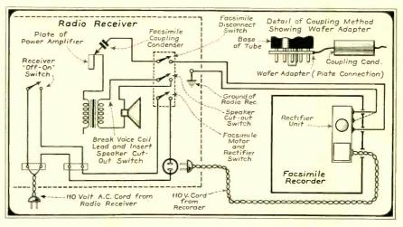
Fig. 1. A facsimile recorder may be connected to the average radio receiver by means of a simple plate connection wafer.
