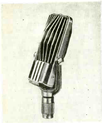
Fig. 1. Velocity mike with directional deflectors.
