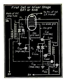
Fig. 2. Superheterodyne mixer stage.
