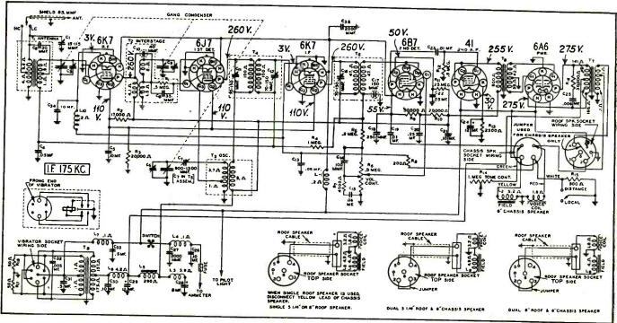
Fig. I. Wells Gardner 6K circuit diagram.
