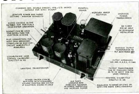
PAK amplifier kits feature: Power output, 35 watts self bias, 55 watts fixed bias; gain 118 DB, immediate change-over to 95 DB; separate power supply and audio decks; stabilized feedback; mobile operation with genemotor—20 watts output; provision for electron mixer or low impedance input if desired.
