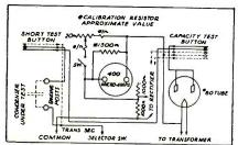
Fig. 1. Breakdown test circuit.
