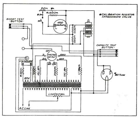
Fig. 4. Triplett 1240 condenser checker circuit.
