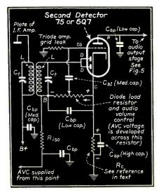
Fig. 4. A simple second detector stage.
