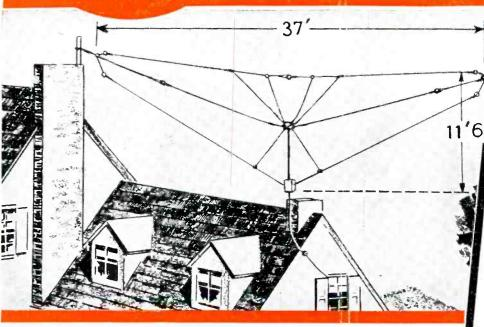
THE RCA Spiderweb Antenna is really five antennas in one. Operates as a T from 140 to 4000 kc., multiple doublet system above to 23,000 kc. With individual antennas for all important short-wave bands, it gives more signals, less noise and better reception on all wave bands. Stock No. 9689 high frequency kit extends coverage to 70 megacycles. This clears up 5-meter complaints that ordinary antennas will not reach.
