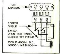
Fig. 4. Phonograph pickup connections.
