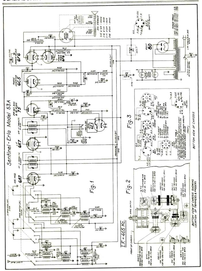
tains two primary coils connected for operation on the "B" band; however, when the band switch is turned to the "C" band position, the lower primary coil, L-5, is shorted out. The high-frequency trimming adjustment, for the "B" band antenna and r-f stages, is accomplished by two adjustable trimmers connected from the "C" band tap on each coil to ground. The capacity coupling coil, L-3, acts only on the "C" band and its function is similar to that of a fixed antenna stage trimmer for that band.
