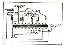
Fig. 3. Transformer circuit Triplett 1240.
