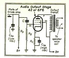
Fig. 5. Typical output stage.
