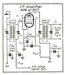
Fig. 3. An i-f amplifier stage.
