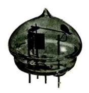
This tube, a filamentary air-cooled triode, is for use by experimenters and amateurs, and is suitable for ultra-high-frequency oscillator and amplifier applications, the frequency limit being 750 megacycles (approx. 0.4 meter).
