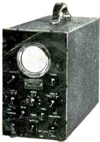
RCA Cathode Ray Oscillograph is entirely self-contained, including power supplies, amplifiers, linear timing frequency generator. Complete with tubes $8450
