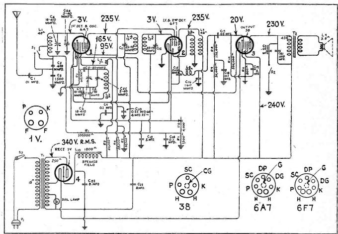
RCA Victor 100 and 101. Note tapped secondary of power transformer
