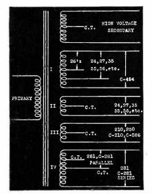
replacement in receivers using such tubes as the '81 half-wave rectifier and 210 amplifier tubes. This transformer also will supply such tubes as the C-484 and C-586 which have 3-volt filaments, as well as the C-210 and one or more '81's in either series or parallel.
