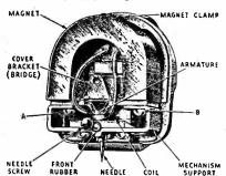
Fig. 1. The parts composing the pickup are marked. Adjustments are made at "A" and "B"
