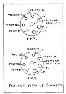
Fig. 3. Socket connections for the Kadette Jr. tubes
