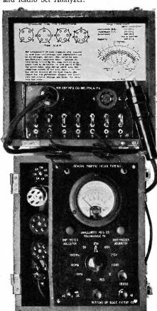
The ranges of this instrument are as follows: D-C Voltage Range (1,000 ohms per volt):—5-25-100-250-1,000 volts. D-C Current Range:—1-10-100-1,000 milliamperes. A-C Voltage Range (1,000 ohms per volt):—5-25-100-250-1,000 volts. Resistance (D-C):—0.5-5,000,000 ohms. Resistance (A.C):—25-3,000,000 ohms. Capacity:—.001-10 mfd. Inductance:—100-10,000 henrys.
