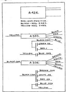
Fig. 4. Coding and connections for the circuit of Fig. 1
