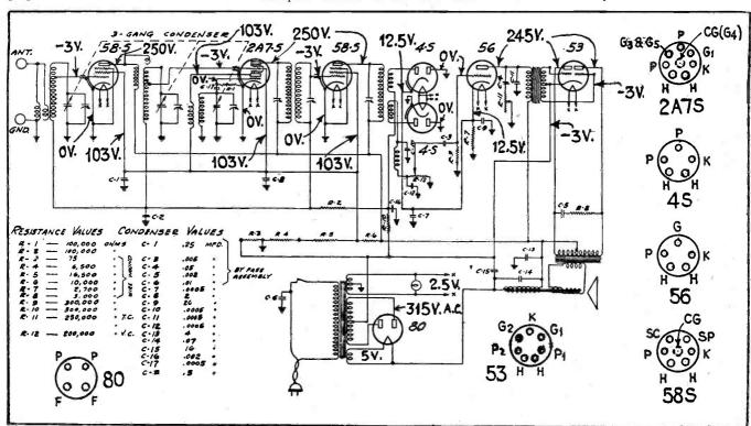
Diagram of the Majestic Model 800 Chassis. Class B is used in the output
