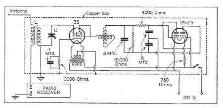
Fig. 3. Complete diagram of the regenerative wave trap
