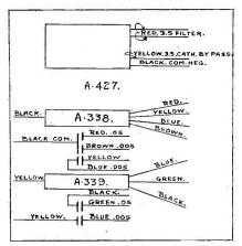
Fig. 5. Coding and connections for the circuit shown in Fig. 2
