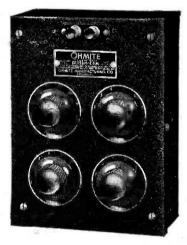
found that the resistor in a receiver has been completely destroyed, and that it is impossible to read the value of the unit or measure it. In such a case, the "Determ-Ohm" is connected in place of the defective resistor and the radio set turned on. The dials on the "Determ-Ohm" should be set at the maximum resistance before the set is operated and then the resistance is gradually reduced until the set functions properly. Then, a glance at the dials shows the proper replacement resistor value.
