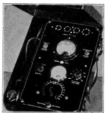
The Franklin Model 33-C English Reading Tube Checker, which uses a single scale meter for all tests. The tube sockets are at the rear
