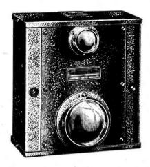
In most devices of this sort the light source is a separate unit. In this device the source of light is included in the case with the photoelectric relay, as will be seen from the accompanying illustration.
