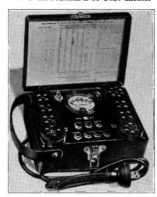
When it comes to tube checking, both instruments are the same, so we shall confine ourselves to a description of the H-33. This unit, it will be seen, has eight sockets mounted on the sides of the panel. These will accommodate all type tubes, including the new 6- and 7-prong tubes. The 7-prong socket will handle tubes with a filament or heater voltage of either 2.5 or 6.3, so that any new tubes which may be an-
