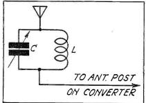
This form of wave trap is satisfactory for the elimination of an interfering signal of broadcast frequency which falls on the i-f. frequency of the shortwave converter. The coil and condenser should be mounted in a shield
