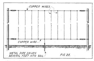
This sketch, and that of Fig. 2D below, give the details of effective "electric curtains." It is seen that they are made up in the form of a wire grid. In both cases the wires represent a single conductor
