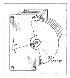
An odd case: The set screw on the rotor shaft became loose and touched the stator section when about 15 degrees below the center, as shown
