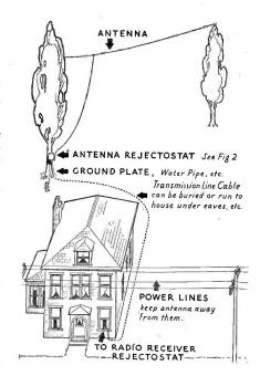
Fig. 2. A typical installation. The aerial should be free of power lines, etc., and free of any obstructions
