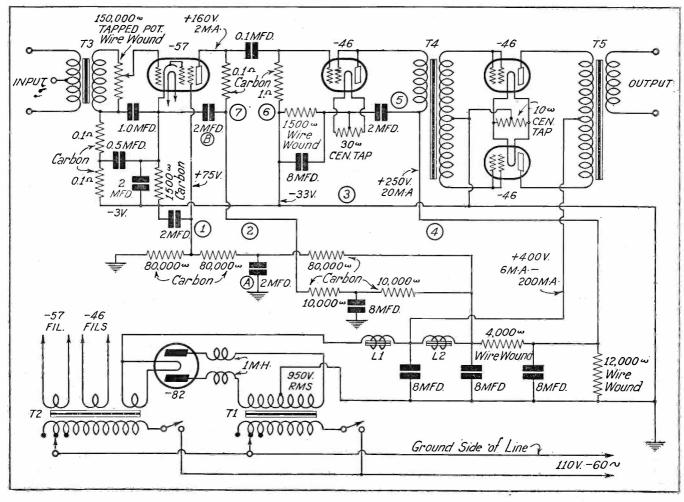
the rectifier (particularly where an 82 is being employed) or other circuit components due to their high impedance and such couplings may be extremely difficult to eliminate.
