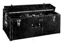
The control panel of the amplifier has provision for microphone, radio and phonograph inputs. Operating switches and volume controls for each input, an amplifier tone control, and all input connections are segregated on this separate unit that may be removed from the amplifier housing when remote control operation is desired. Extension cables up to 500 feet in length may be used without affecting the operation of the amplifier.
