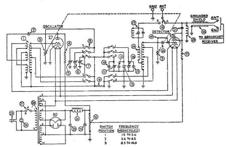
Schematic diagram of the Philco 4 and 4C Short Wave Converter. The numbers in this diagram correspond to the numbers on the chassis and in the parts list on the opposite page. The voltage data for the three tubes is given in Table 1
