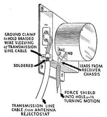
Fig. 4. The Receiver Rejectostat. This unit is mounted in the receiver cabinet. Be sure the shield is replaced over the aerial and ground leads
