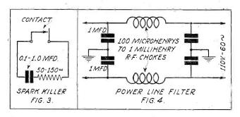
The arrangement shown in Fig. 3 is effective for most any type of make-and-break circuit. The circuit of Fig. 4 will quell line surges
