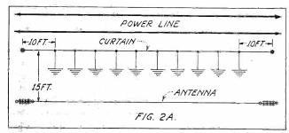
An antenna can be shielded from power-line interference by the use of an "electric curtain." Details of such curtains are given in Figs, 2E and 2D
