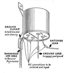
hang from the Antenna Rejectostat. It should be tied off to several supports on the way down to the receiver.
