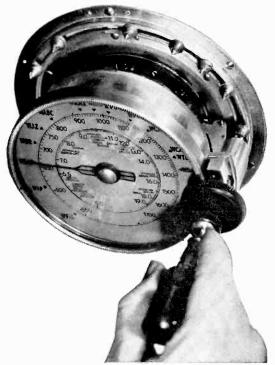
Fig. 2—Tuning Handle and Wrench Engaging stop
