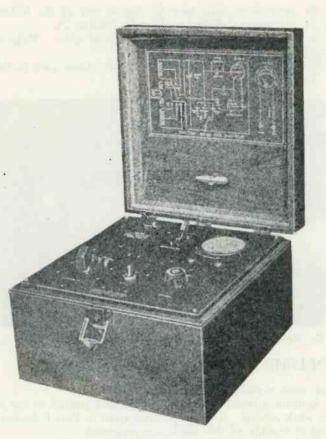
Figure 9-180 K.C. Test Oscillator
