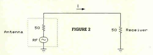
Thevenin equivalent circuit of an antenna feeding a receiver with proper impedance match for maximum energy transfer. Only 50 percent of the energy received by the antenna is delivered to the receiver. The rest is re-radiated back into space by the antenna.
