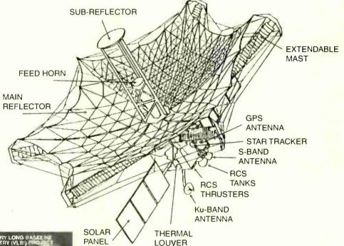
Telescope at optical wavelengths. The satellite's resolving power is equivalent to being able to see a grain of rice in Tokyo from Los Angeles.
