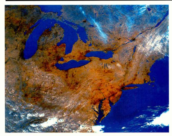
Section of a multi-spectral, false-colorized NOAA APT image of the Northeast US. This image was created directly from a raw image file using the MFCOLOR software from Weather Dynamics.
