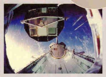
There's no substitute for experience, and from its inception the Long-Duration Exposure Facility (LDEF) was employed as the ultimate orbital guinea pig, performing 87 experiments to gauge the long-term effects of space travel—not the least of which were tests on the space-worthiness of various structural materials.
