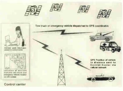
**FIGURE 1**: Using GPS to locate a driver in distress and dispatch the nearest break-down or emergency assistance
