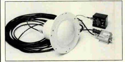
The Integrated Feed Antenna/ LNA/Down Converter is ready to mount on our Model WPDA-3 Dish. A mounting ring is drilled to accommodate the 3 strut mount. Unit is powered by a bias-T/ regulator which splits off the 137.5/137.1 MHz IF to a BNC output connector while routing regulated +15 VDC up the coax cable.
