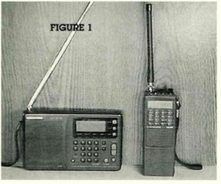
Simple Mode A CW ground station consisting of a Grundig YB-400 portable shortwave receiver and Radio Shack HTX-202 2-meter handheld transceiver. Such a combination is effective for making portable CW contacts through RS-10's Mode A ROBOT.
