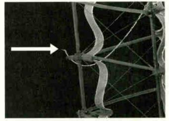
The frayed end of the tether portion of the Tethered Satellite System (TSS) is seen at the end of the supportive boom. On February 25, 1996, the STS 75 crew deployed the TSS, which later broke free.
