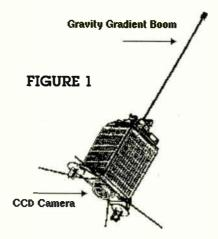
Drawing of the UoSAT-OSCAR-11 spacecraft. Notice the CCD imaging camera at the base of the satellite. A gravity gradient boom at the top of the spacecraft is used to keep the camera pointing toward the earth.
