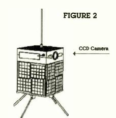
The WEBERSAT-OSCAR-18 microsat satellite. A color CCD video camera is mounted towards the top of the spacecraft. Passive attitude control (a simple bar magnet) aligns the satellite with the earth's magnetic field, allowing the camera to point toward the surface of the earth.
