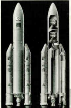
Above, cross-sectional view of the the Ariane-5 launcher reveals the rocket's internal configuration for its doomed maiden flight with the four indentical CLUSTER satellites.
