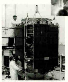
The NEAR satellite under construction and the Delta II rocket that put it in space.
