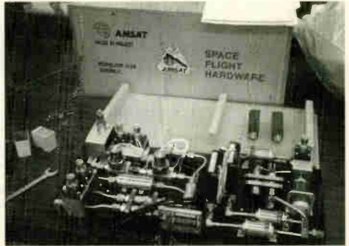
Student project co-leaders Gene Hansen (left) and Richard Vanderford (right) inspect the completed flight model Phase 3D SBS in the P3D lab at Ogden, Utah. The SBS will be used to carry the spacecraft into orbit aboard its Ariane 5 launch vehicle.
