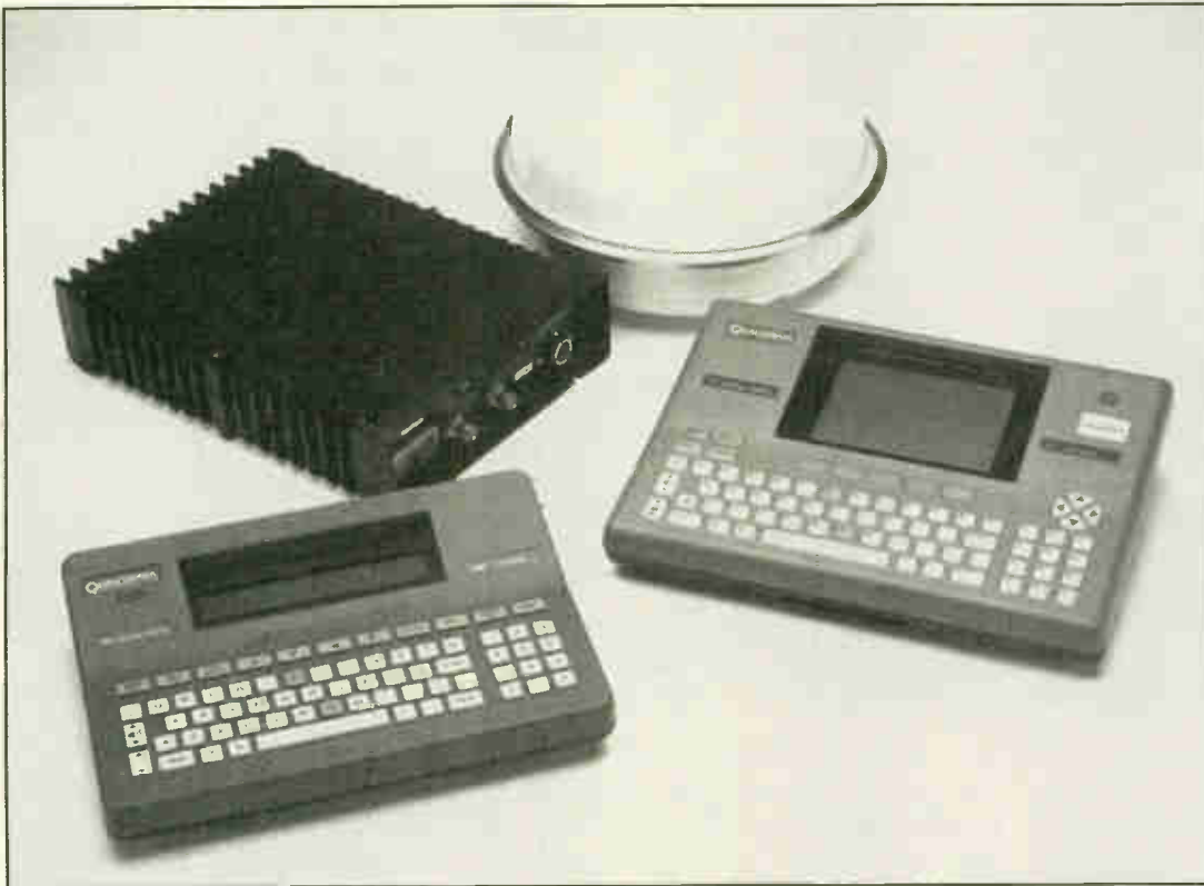
Three hardware components comprise the OmniTRACS Mobile Communications Terminal (MCT). The optional enhanced display unit (right) features a 15-line by 40-character screen that permits both text and high definition graphics.
