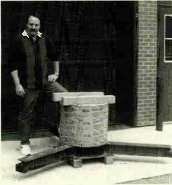
Jaim Parsons, Weber State University, poses with the Phase 3D Mass Mockup Unit (MMU) outside the P3D laboratory in Ogden, Utah. Made from over 495 kg (1,100 lbs) of concrete and steel, this ungainly apparatus simulates the exact weight and balance characteristics of a fully configured Phase 3D spacecraft. During recent tests, also done at Weber State, the MMU was successfully used to verify that the Phase 3D spacecraft should separate "cleanly" from its Specific Bearing Structure (SBS) carrying structure during launch.
