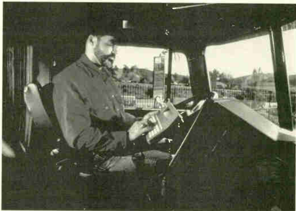
In-cab communications using the OmniTRACS system ensures that drivers are never out of touch. The user-friendly keyboard prompts the operator with simple, straight forward language and commands.
