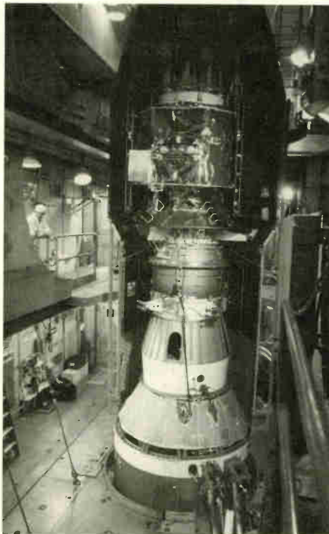
Delta GPS-25, Navstar II-12 installation of the fairing at complex 17B at Cape Canaveral Air Station. (U.S. Air Force photo)
