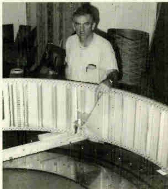
Jaim Parsons, Weber State University, poses with the Phase 3D Mass Mockup Unit (MMU) outside the P3D laboratory in Ogden, Utah. Made from over 495 kg (1,100 lbs) of concrete and steel, this ungainly apparatus simulates the exact weight and balance characteristics of a fully configured Phase 3D spacecraft. During recent tests, also done at Weber State, the MMU was successfully used to verify that the Phase 3D spacecraft should separate "cleanly" from its Specific Bearing Structure (SBS) carrying structure during launch.
