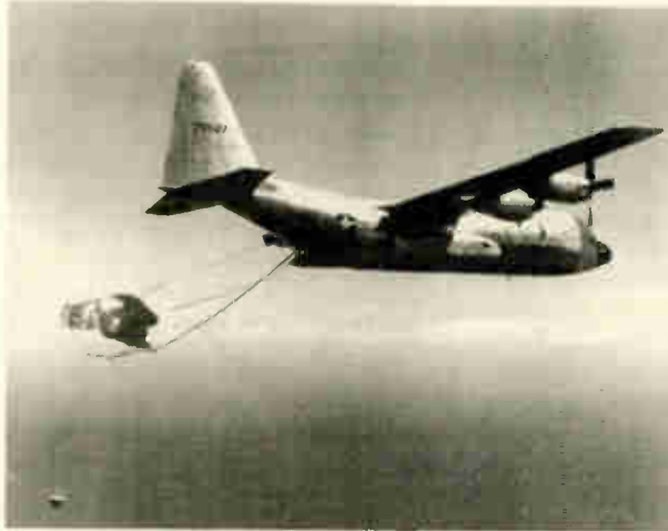
A U.S. Air Force JC-130A modified with poles, lines and winches extending from the rear cargo door captures a capsule ejected from a Discoverer satellite. the same aircraft were used to retrieve Corona film capsules.
