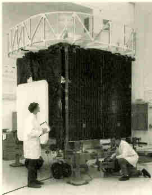
The U.S. Navy's UHF Follow-On F-3, undergoes mass property testing in El Segundo, Calif. (Photo courtesy of Hughes Space and Communications)
