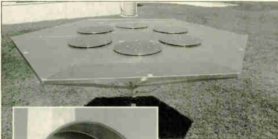
Above: The flight prototype U-band patch array undergoes testing on the Phase 3D integration facility antenna range. The array exhibits gain figures comparable to that of a commercial 40 element crossed yagi antenna. Actual on-the-air contacts, with surprisingly good results, have been made through the AMSAT Oscar 13 satellite using this array as an uplink antenna.
