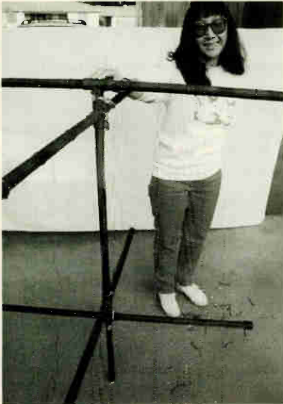
Satellite enthusiasts Jade Smith shows the completed turnstile antenna. In theory, both pickup/reflector pairs should be equidistant. Putting one pair closer together eliminated an annoying "null" in the pickup pattern when the satellite was directly overhead. (Photo by Raymond Smith)
