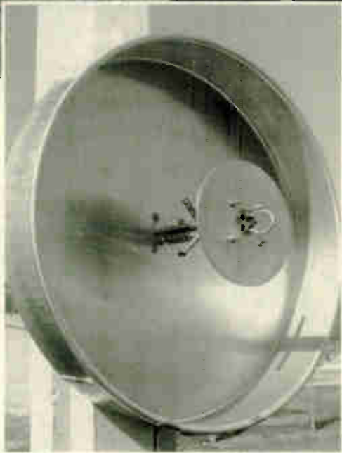
Above: The completed Phase 3D flight model L-band antenna undergoing gain and pattern testing at the integration facility's antenna test range. Preliminary gain measurements exceeded 15 dBic with a surprisingly clean pattern. The antenna is based on a short-backfire design and uses an all-aluminum wedding cake baking pan for a reflector!
