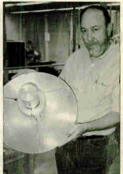
Above: Mike Garrity, N4OZC, displays a flight model prototype of Phase 3D's S-band antenna.
