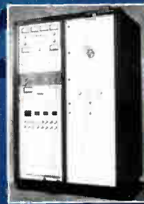
11 kW FM Transmitter
