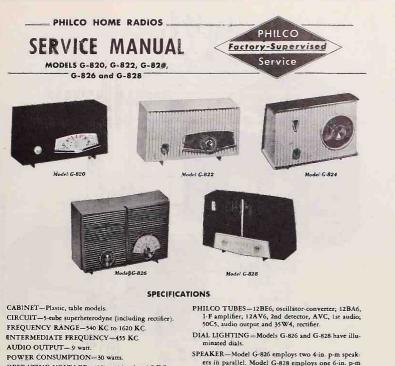
OPERATING VOLTAGE-105 to 125 volts, AC-DC. AERIAL-High Impedance loop mounted on inside of back. SPEAKER—Model G-826 employs two 4 in. p-m speakers in parallel. Model G-828 employs one 6 in. p-m speaker and one 4x6 in. p-m speaker connected in parallel. The others use one 4 in. p-m speaker.
