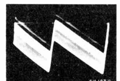
Figure 44—Horizontal (7.5 Volts PP)
