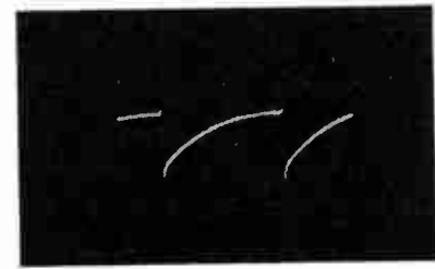
Fig. 13. Vertical-Oscillator Grid, Pin 7, 140 volts, 60 c.p.s.
