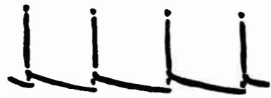
PIN 9 (V15) 6S4 VERTICAL OUTPUT 850 VOLTS PP
