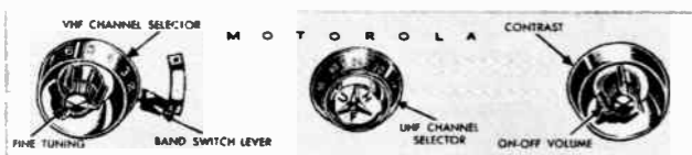
VHF-UHF Receiver Controls
