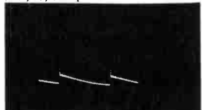
Fig. 15. Vertical Output Plate, Pin 9, 1100 volts, 60 c.p.s.
