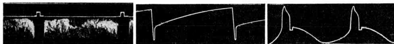
No. 2—12AT7 Plate 44V P-P 60 C.P.S. No. 2—12BY7 Grid 9.5V P-P 60 C.P.S.
