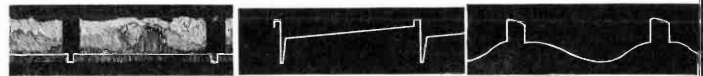
No. 3—Pix Tube Grid 20-100V P-P 60 C.P.S.
