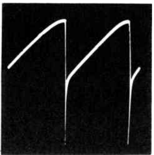
V-106B Vert. Out. Grid Pin 7 Sweep Freq. 30 cps Voltage P/P 90 volts
