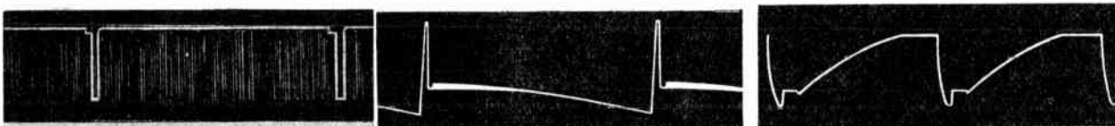
No. 5—6CS6 Sync Sep. Plate 36V P-P 60 C.P.S.
