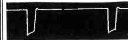
No. 6 -- 12A77 Phase Splitter Cathode 18V P-P 15,750 C.P.S.
