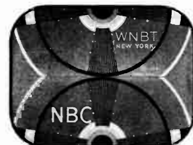
IF PATTERN continuously rolls across screen in vertical direction (up or down) ADJUST VERTICAL HOLD CONTROL so that pattern stops rolling and remains stationary on screen.
