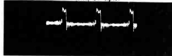
Figure 16. Gated-Leveler Grid, Pin 2, 3 volts, 15,750 c.p.s.
