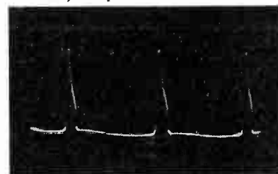
Fig. 18. Horizontal-Oscillator Cathode, Pins 3 and 8, 18 volts, 15,750 c.p.s.
