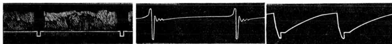
No. 3—Pix Tube Grid 23-150V P-P 60 C.P.S.
