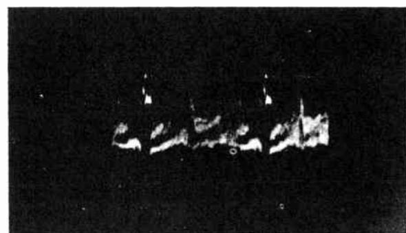
Figure 13. Sync Separator Grid, Pin 7 40 volts, 60 c.p.s.
