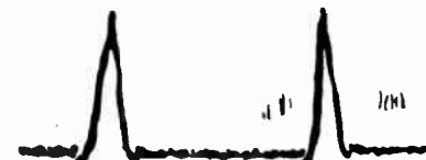
PIN 6 (V9B) 12AU7 SYNC. CLIPPER (HORIZ. SCOPE) 65 VOLTS PP
