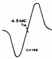
Figure 21 Ratio Det. Response
