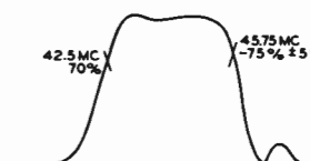
Figure 9—KRK22D T1 and T104 Response
