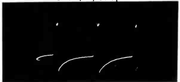
Figure 34. Horizontal-Deflection Yoke, Pin 7 of J800 5600 volts, 15,750 c.p.s.
