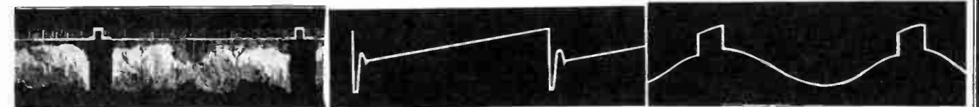
No. 2—12AT7 Plate 35V P-P 60 C.P.S. No. 2—6AH6 Grid 8V P-P 60 C.P.S.
