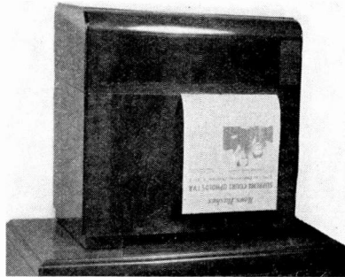
A newspaper printed by the RCA facsimile receiver coming from the cabinet.
