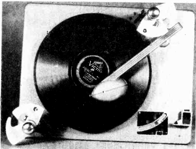
FIG. 7. Start of vertical motion of tone arm to lift pick-up from the record. This is check point No. 4.
