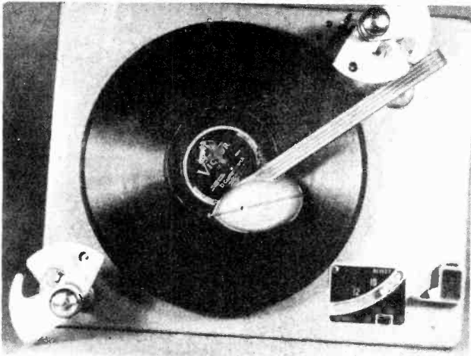
FIG. 5. The pick-up has reached the end groove of the record, which shifts trip mechanism (see Fig. 6) to start record-changing cycle. This is check point No. 3.
