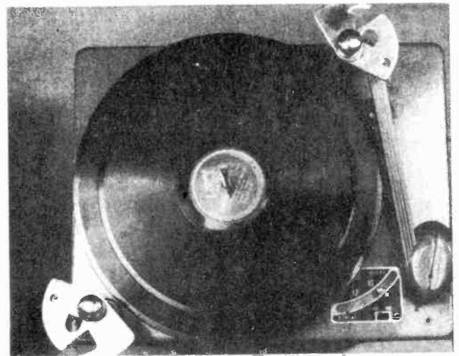
FIG. 28. This shows the tone arm in the rest position with the record shelves have been swung outwards manually so that the played records on the turntable can be removed.
