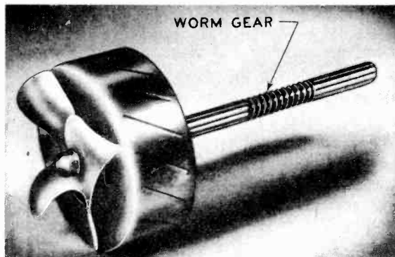
FIG. 30. A worm gear has been cut in the shaft of the rotor of this commercial motor. This worm drives the turntable through a gear on the turntable shaft. See C and D of Fig. 35.
