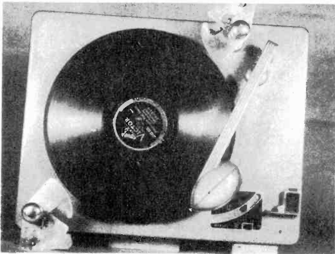
FIG. 15. The tone arm has returned to a position just over the outer rim of unplayed record. Record shelves have just started to return to their normal positions. This is check point No. 8.
