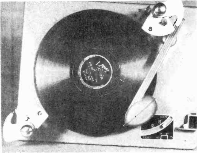
FIG. 1. The pick-up needle is in the outer groove preparatory to the playing of the record. The record supporting shelves are in their normal position to support a stack of 10-inch records. This is check point No. 1.
