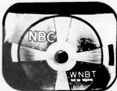
FOCUS COIL & ION TRAP MAGNET REQUIRES ADJUSTMENT
