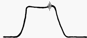
RESPONSE GOOD, BUT RESONANT FREQUENCY OF TUNED CIRCUIT A LITTLE LOW
