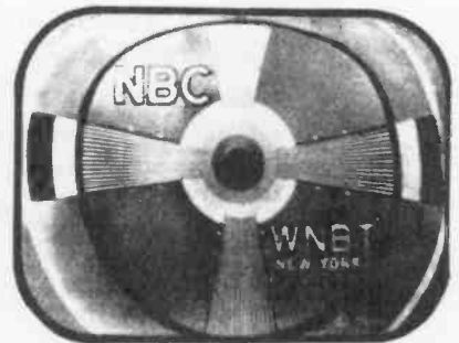
VERTICAL LINEARITY CONTROL REQUIRES ADJUSTMENT
