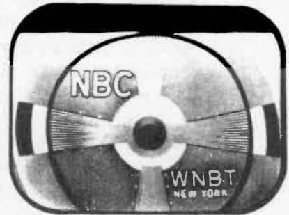
VERTICAL CENTERING CONTROL REQUIRES ADJUSTMENT
