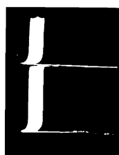
10 1100 volts p/p, total, ±20 volts p/p sawtooth, 60 cps
