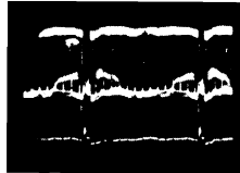
2 2.5 volts p/p, 60 cps (max. contrast)
