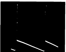
11 80 volts p/p, total, 180 volts p/p sawtooth, 60 cps
