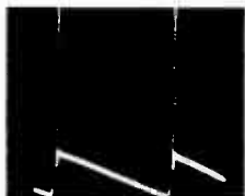
16 620 volts P/P total, 250 volts P/P sawtooth, 60 CPS
