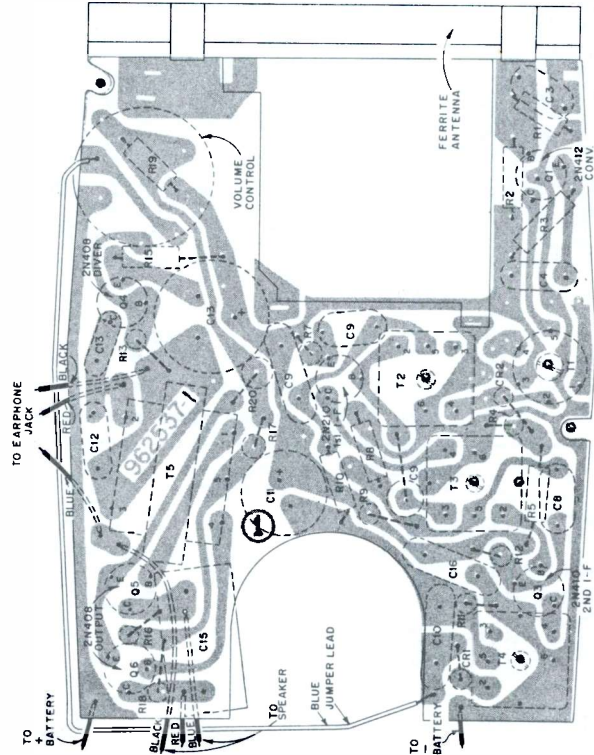
Wiring and Components — View from Wiring Side
