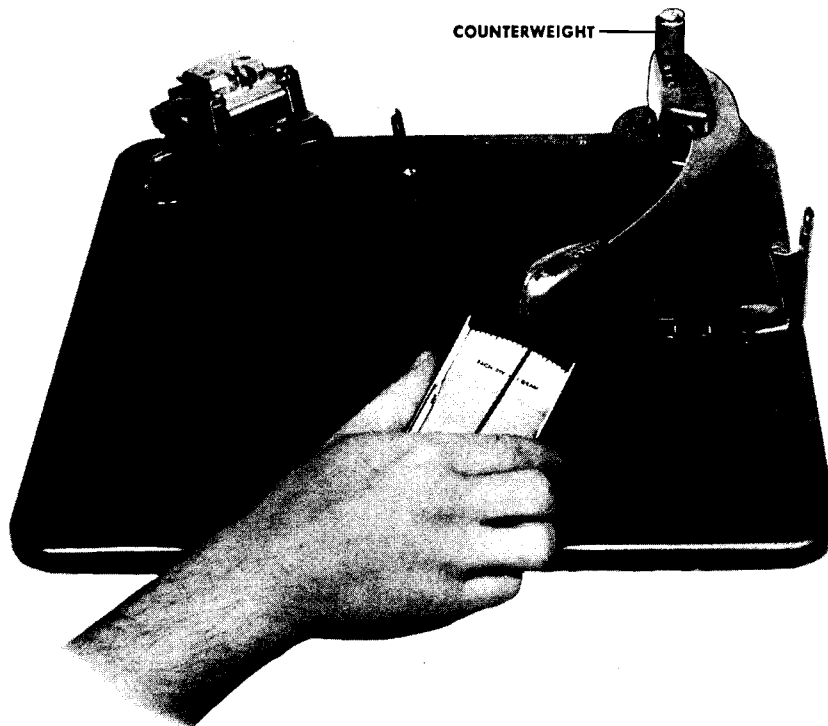
FIGURE 10. MEASURING HORIZONTAL FRICTION
