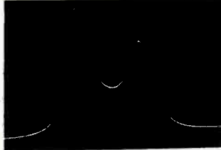
Figure 15-B Oscilloscope of the single sound IF curve (untuned). This is the response curve appearing on the right of Figure 15-A after it has been expanded.
