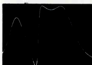
Figure 15-X Video IF response curve: Wobbulator to the grid of V11 and the travelling detector to the oscillograph at the plate of V12. L27 and L28 properly tuned (birdie at 26.4 mc.).
