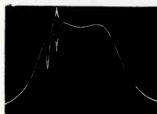
Figure 15-U Sound trap much too low. Birdie at 21.9 mc.
