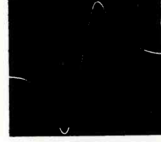
Figure 15-L Properly aligned discriminator curve. Birdie at 21.9 mc.
