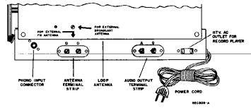
Fig. 3. Antenna & record player connections
