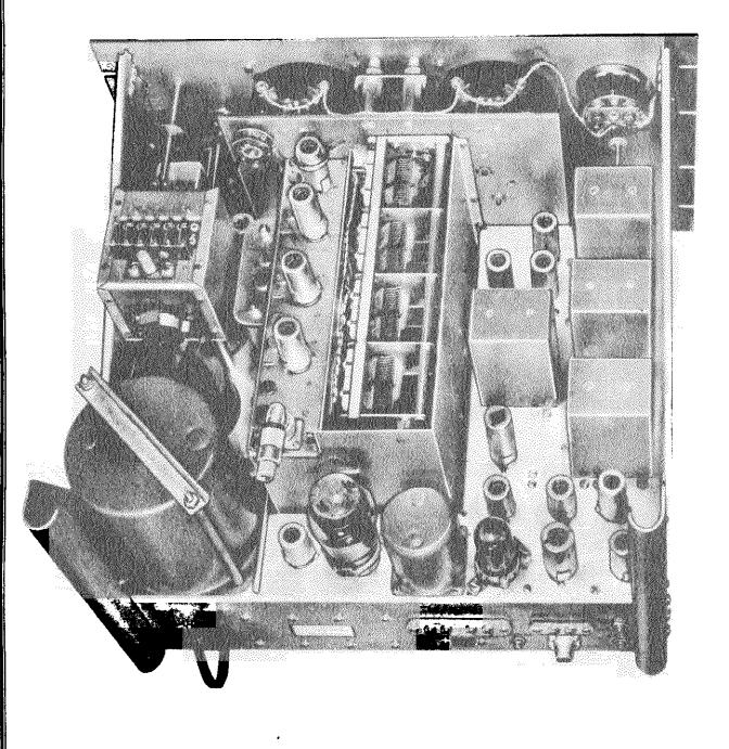
FIG. 8 TOP VIEW OF RECEIVER CAPACITOR SHIELD REMOVED
