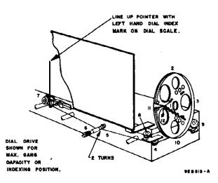
Fig. 4. Dial cable stringing procedure
