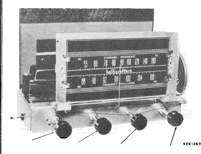
This is a combinatio power switch and tone con trol. In the OFF position the receiver is complete turned off. To turn on th receiver, turn the control to the right. The powe switch will click and th dial light will illuminat the dial face indicating that the receiver is receiving clockwise to depower from the wall outlet. After tuning in the crease volume. station this control is again adjusted for the desired tonal response. Turning the control clockwise decreases the bass response.
