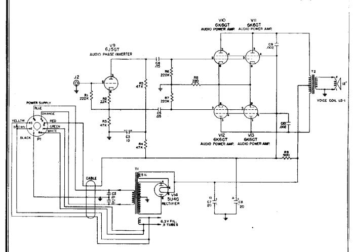
Figure 8. Schematic Diagram of Power Supply and Audio Section
