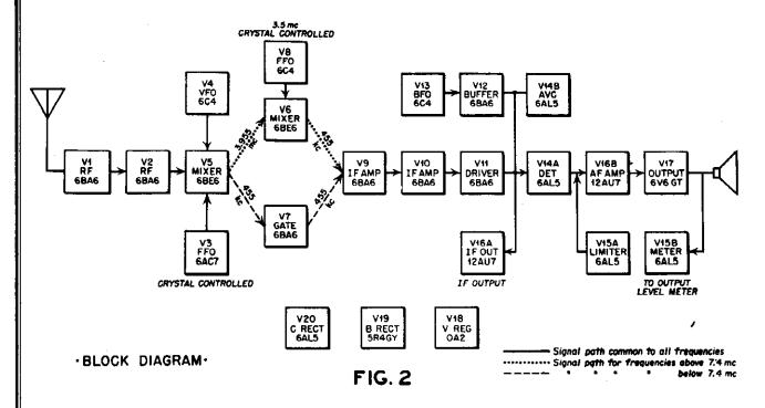
switch S-6, permits optional use of the limiter on any mode of operation when pulse type interference is present.
