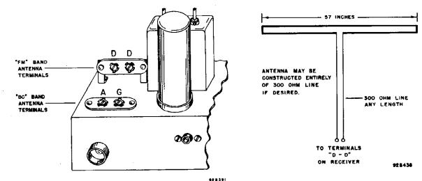
Pig. 2. Antenna terminal strip connections Fig. 3. Polded doublet antenna details.
