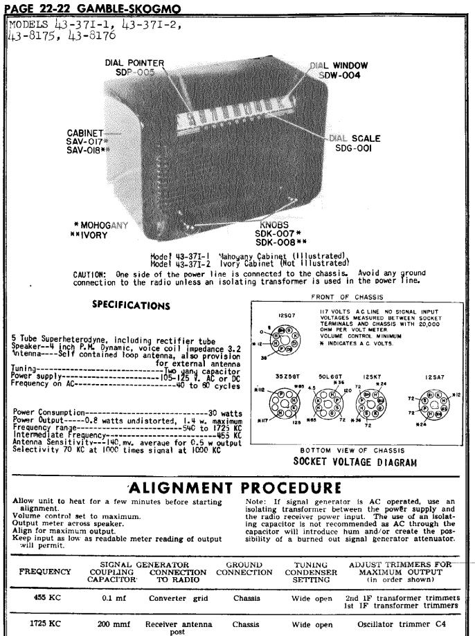
200 mmf Receiver antenna Chassis Tune for Antenna trimmer C2 post maximum output
