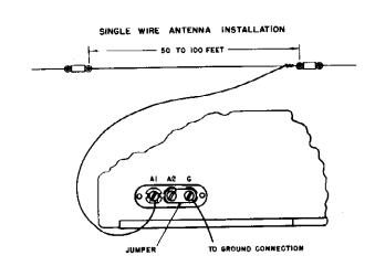
SINGLE WIRE ANTENNA - For a single wire antenna installation, connect a jumper between antenna terminals "A2" and "G". A single wire antenna of about 50 to 100 feet long (including lead-in) is then connected to terminal "A1". Erect the antenna as high and free of surrounding objects as possible. For improved reception, it may be desirable to connect a ground wire between terminal "G" and a suitable ground such as a water pipe or outside ground stake.
