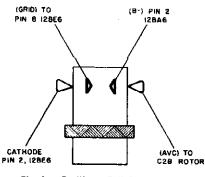
Fig. 1. Oscillator Cail Connections
