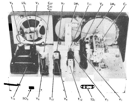
Fig. 4. Top view, component location
