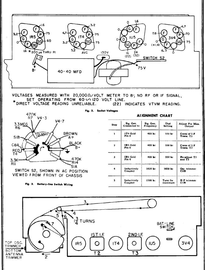
Fig. 4. Dial Stringing and Tube and Trimmer Location
