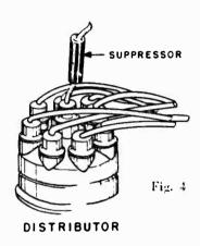
Disconnect the high tension wire that runs from the ignition coil to the center hole of the distributor cap. Cut lead one inch back from the metal tip end. Screw suppressor into cut end of long lead. Screw cut end of short lead into suppressor. Plug lead with attached suppressor back into distributor cap.
