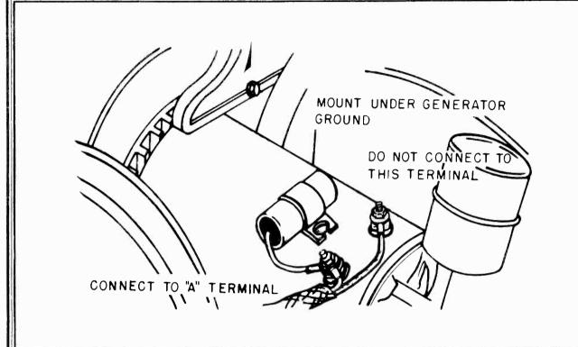
FIG. 2 GENERATOR CONDENSER
