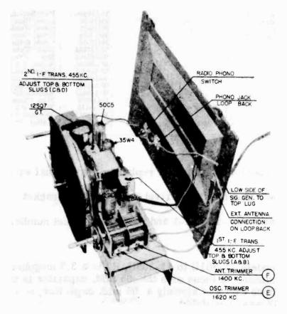
CHASSIS, TOP VIEW (Sets equipped with 12AV6 Tube)
