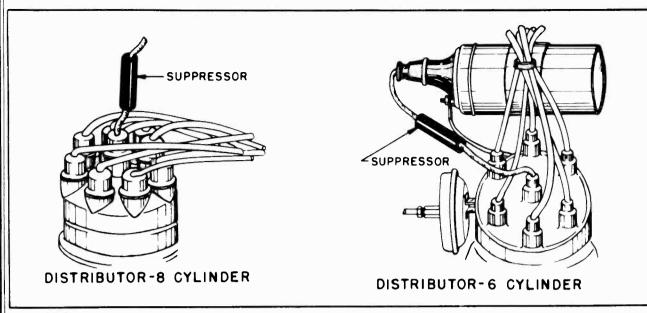
FIG. 2 DISTRIBUTOR SUPPRESSOR
