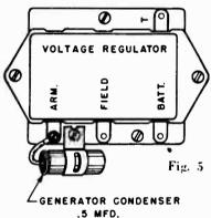
Loosen voltage regulator mounting screw. Insert slotted end of generator condenser mounting bracket under this screw and tighten screw. Connect condenser lead to armature terminal marked "ARM."
