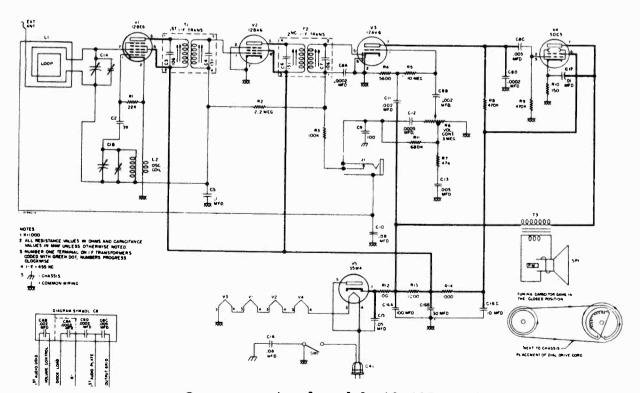
On some sets of models 10-135 to 10-140, R2 is a 3.3 megohm, 10%, 1/2 watt resistor instead of a 2.2 megohm resistor; and because of this C5 is an .05 mfd., 600 volt paper capacitor (Part No. 39001-17).
