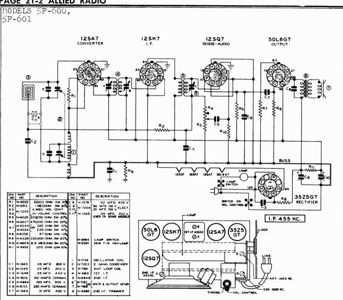
This receiver is designed to operate over the standard broadcast band which extends from 535 to 1620 Kilocycles (KC) (185 to 560 Meters.)
