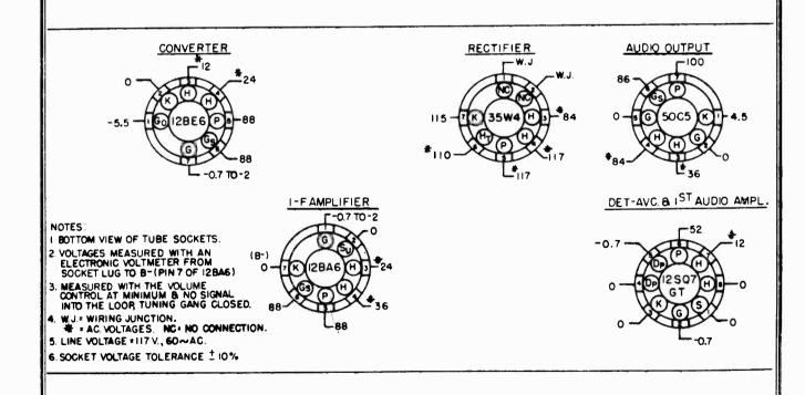
SOCKET VOLTAGE CHART (Sets equipped with 12SQ7GT Tube)
