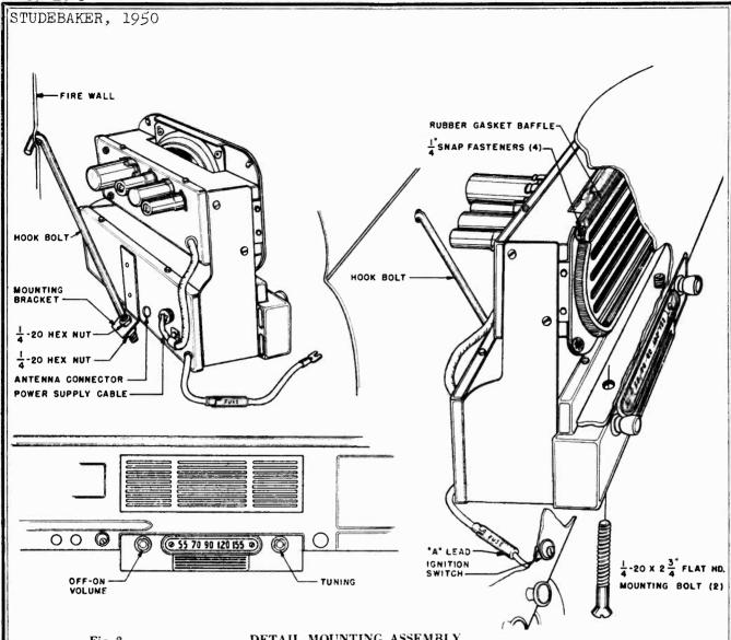
Fig. 2 MOUNTING PARTS KIT
