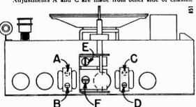
Trimmer Location, Underside of Chassis
