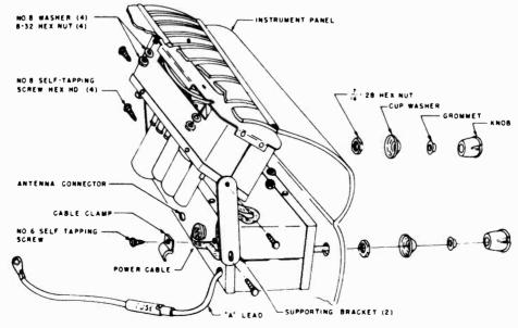
FIG. 1 DETAIL MOUNTING ASSEMBLY
