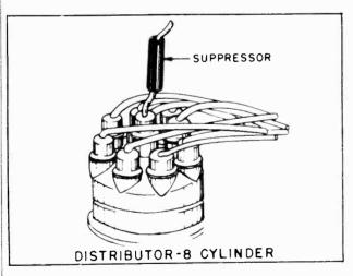
FIG. 3 DISTRIBUTOR SUPPRESSOR
