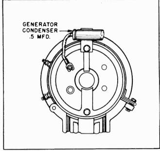
FIG. 3 GENERATOR CONDENSER
