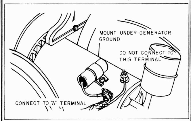
FIG. 2 GENERATOR CONDENSER
