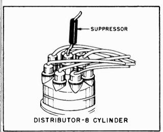
FIG. 3 DISTRIBUTOR SUPPRESSOR
