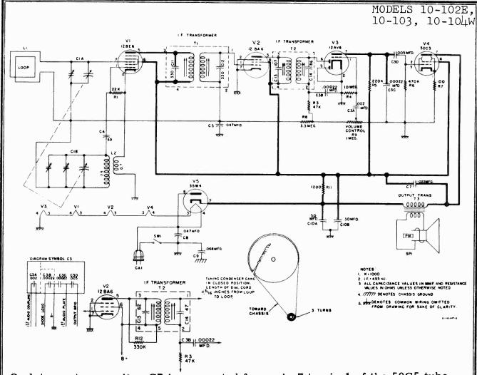
On later sets capacitor C7 is connected from pin 7 to pin 1 of the 50C5 tube instead of across the primary of the output transformer. This will improve stability.
