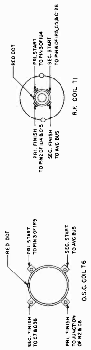
Fig. 7. Coil and Switch Terminal Identification
