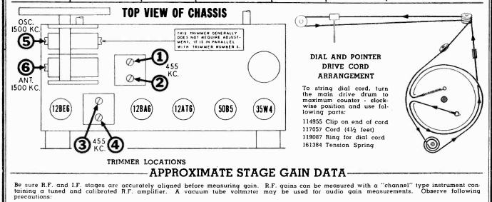
For all gain measurements connect signal generator as shown. Use 600 KC. signal with 400 cycle modulation (use nearby frequency if local station interferes.) 2. For R.F. and I.F. measurements connect negative terminal of a 3 volt battery (two  $1\frac{1}{2}$  volt cells in series) to A.V.C. connection at loop antenna (white wire) and connect positive battery terminal to  $B_{--}$ . This provides a definite operating point.
