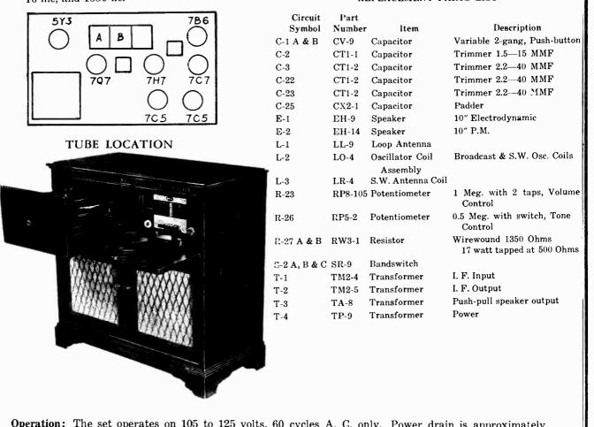
**Operation:** The set operates on 105 to 125 volts, 60 cycles A. C. only. Power drain is approximately 70 watts for the radio and about 20 watts additional for the record changer.
