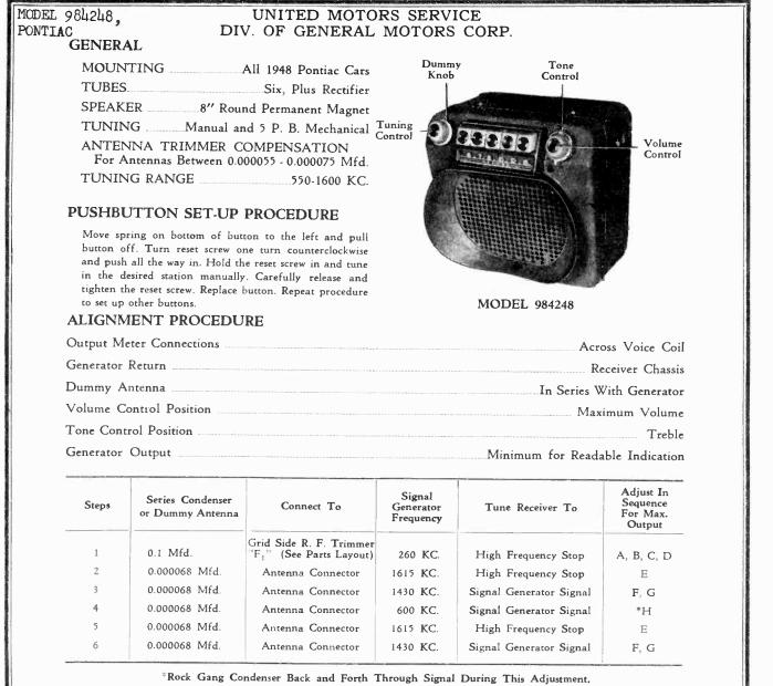
With the Radio Installed and the Car Antenna Plugged In Adjust the Antenna Trimmer "G" for Maximum Volume With the Radio Tuned To a Weak Station Near 1400 KC. (See Sticker On Case).
