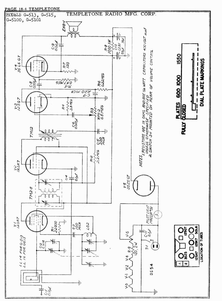
radio is a 5-tube super-heteroodyne receiver using the latest type of low-drain electronic tubes.
