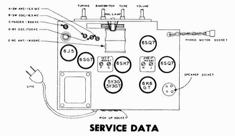
Lack of sensitivity and poor tone quality may be due to any one or a combination of causes such as weak or defective tubes or speaker, open or grounded bias resistor, bypass condenser, etc. Never attempt to realign set until all other possible sources of trouble have been first thoroughly investigated and definitely proved not to be the cause.
