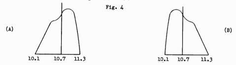
Now if this overcoupled circuit is combined with a single peaked circuit (where the coupling is below critical) the misalignment becomes worse, something like Fig. 5.
