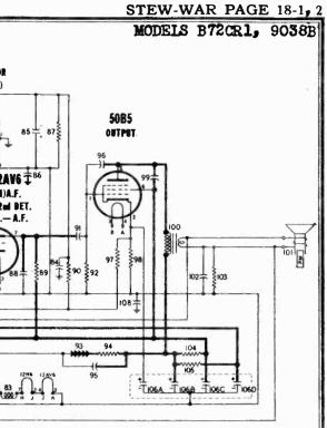
or if the feed-back connection is made to the wrong side of the output transformer secondary, the system will become regenerative instead of degenerative. Under those conditions audio oscillation may result. If that occurs, oscillation may be prevented by reversing the connections to the secondary of the output transformer.
