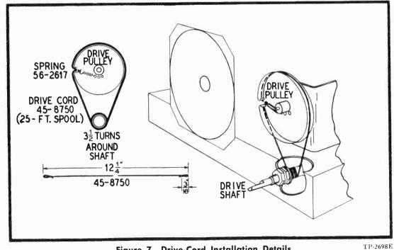
Figure 7. Drive-Cord Installation Details
