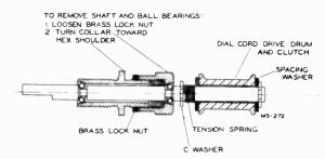
SOME MODELS MAY HAVE EXTRA SPACING WASHER TO INCREASE CLUTCH FRICTION
