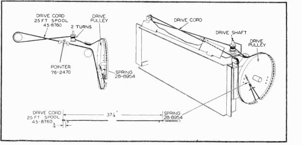
Figure 7. Drive-Cord Installation Details
