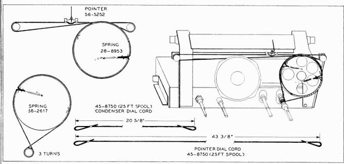
Figure 5. Drive-Cord Installation Details
