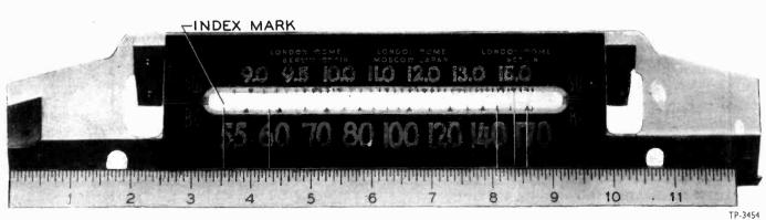
FIGURE 6. COMPOSITE DIAL AND BACKPLATE, CALIBRATION DETAILS.
