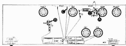
Figure 1. Bottom View, Showing Section 1 Test Points
