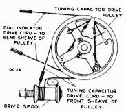
END VIEW OF DRIVE MECHANISM SHOWN WITH TUNING CAPACITOR AT MAX. CAPACITY.
