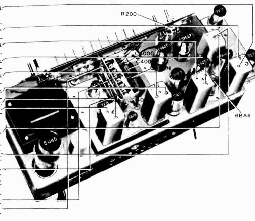
Figure 9. Top View, Showing FM Trimmer Locations
