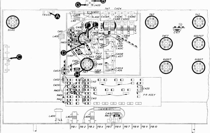
Figure 5. Bottom View, Showing Section 4 Test Points
