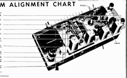
NOTE: Make up a six-to-eight-turn, 6-inch-diameter loop, using insulated wire; connect to the signal-generator leads and place near the radio loop.
