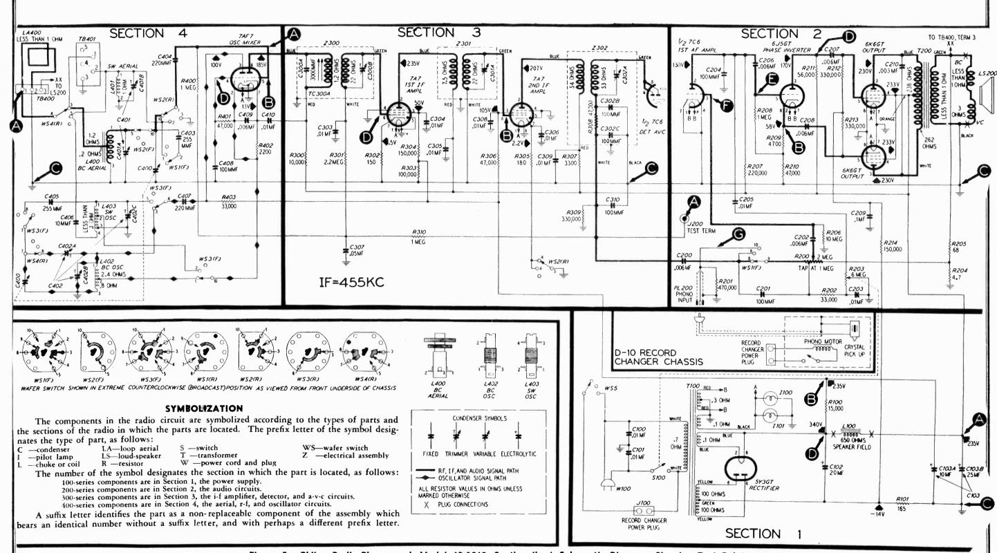
Figure 5. Philco Radio-Phonograph Model 48-1263, Sectionalized Schematic Diagram, Showing Test Points
