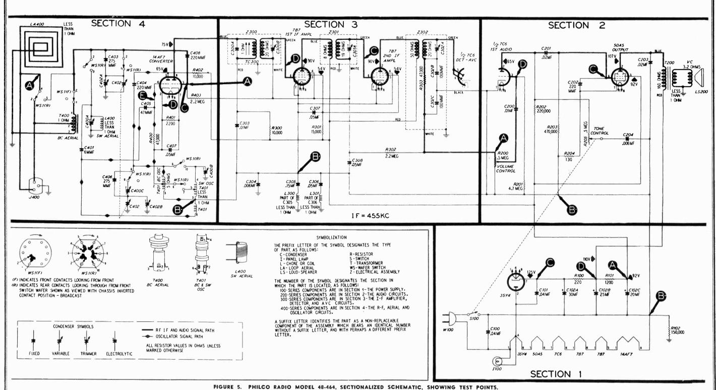
Source 3. Philod Rabid Mobel 40-404, Sectionalized Schematic, Showing 1251 Points.
