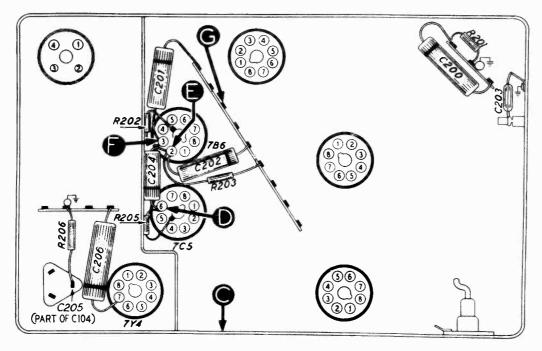
Bottom view, showing Section 2 test points.
