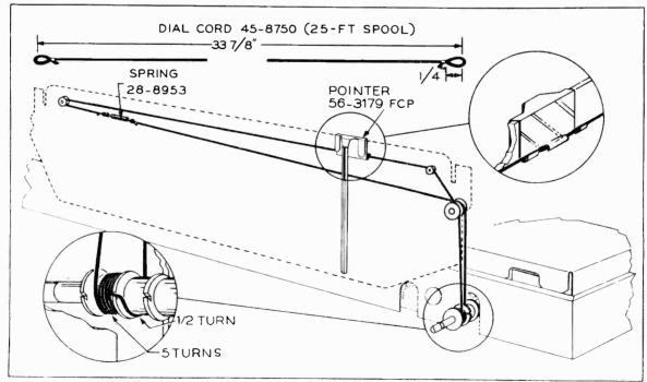
Figure 7. Drive-Cord Installation Details
