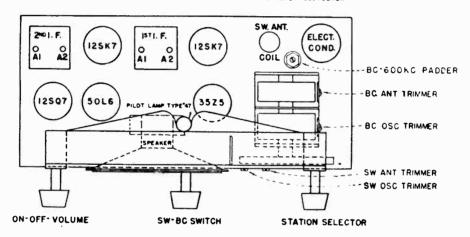
This Model is a 5 tube 2 band superheterodyne which will give reception over a wide range, including standard broadcast and foreign shortwave. The tuning range of the broadcast frequency is 540 to 1650 kilocycles, or 560 to 182 meters. The short wave frequency is 5.8 to 18.3 megacycles, or 16 to 49 meters, which includes the following: 16, 19, 25, 31, 39 and 49 meter bands.
