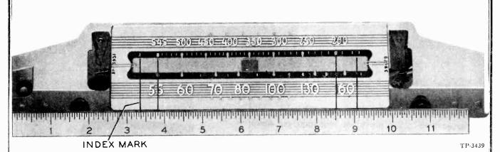
Figure 8. Composite Dial and Backplate, Calibration Details
