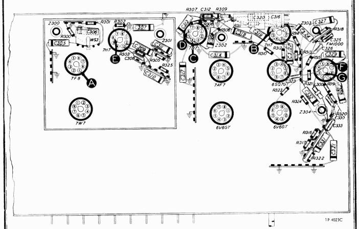
Figure 4. Bottom View, Showing Section 3 Test Points
