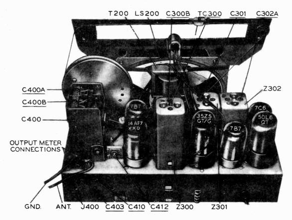
Figure 11. Top view, showing trimmer condenser locations.
