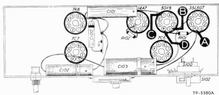
1. Bottom View, Showing Section 1 Test Points
