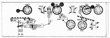
FIGURE 3. BOTTOM VIEW, SHOWING SECTION 3 TEST POINTS.
