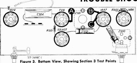
Make tests for this section by using an r-f signal generator with modulated output. Set generator frequency to 455 kc. Connect ground lead of signal generator to B—; connect output lead through a .1-mf condenser to the test points indicated in the chart. Set the volume control at maximum. If "NORMAL INDICATION" is obtained in step 1, proceed with tests for Section 4; if not, isolate and correct the trouble within this section.
