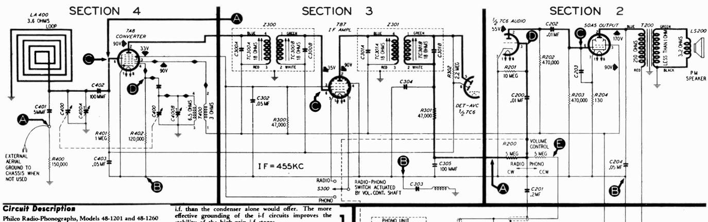
are identical electrically. The radio is a five-tube superheterodyne with a built-in loop aerial and provisions for connecting an external aerial.
