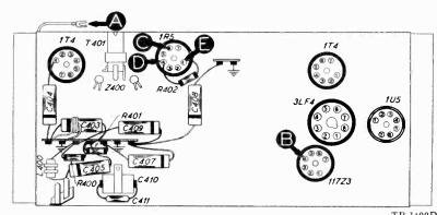
Figure 4. Bottom View, Showing Section 4 Test Points (Locations of C402 and T400 shown in figure 6.)
