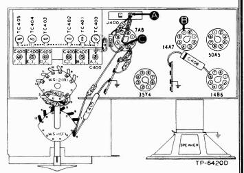
Figure 4. Bottom View, Showing Section 4 Test Points
