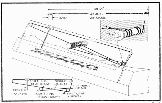
Figure 6. Drive-Cord Installation Details
