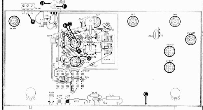
BOTTOM- VIEW, SHOWING SECTION 5 TEST POINTS.
