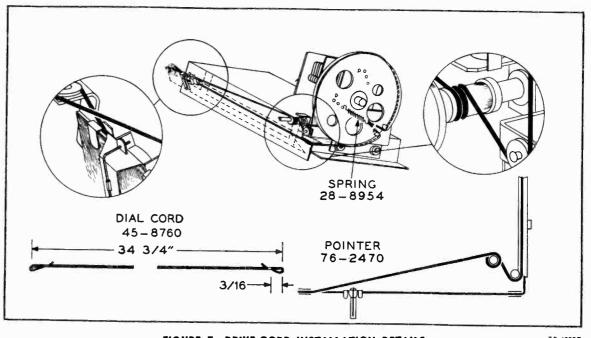
FIGURE 7. DRIVE-CORD INSTALLATION DETAILS
