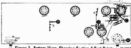
Figure 2. Bottom View, Showing Section 2 Test Points
