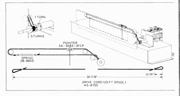
Figure 8. Drive-Cord Installation Details
