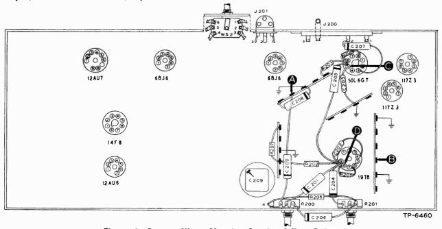
Figure 2. Bottom View, Showing Section 2 Test Points
