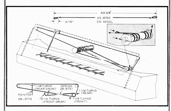
Figure 6. Drive-Cord Installation Details
