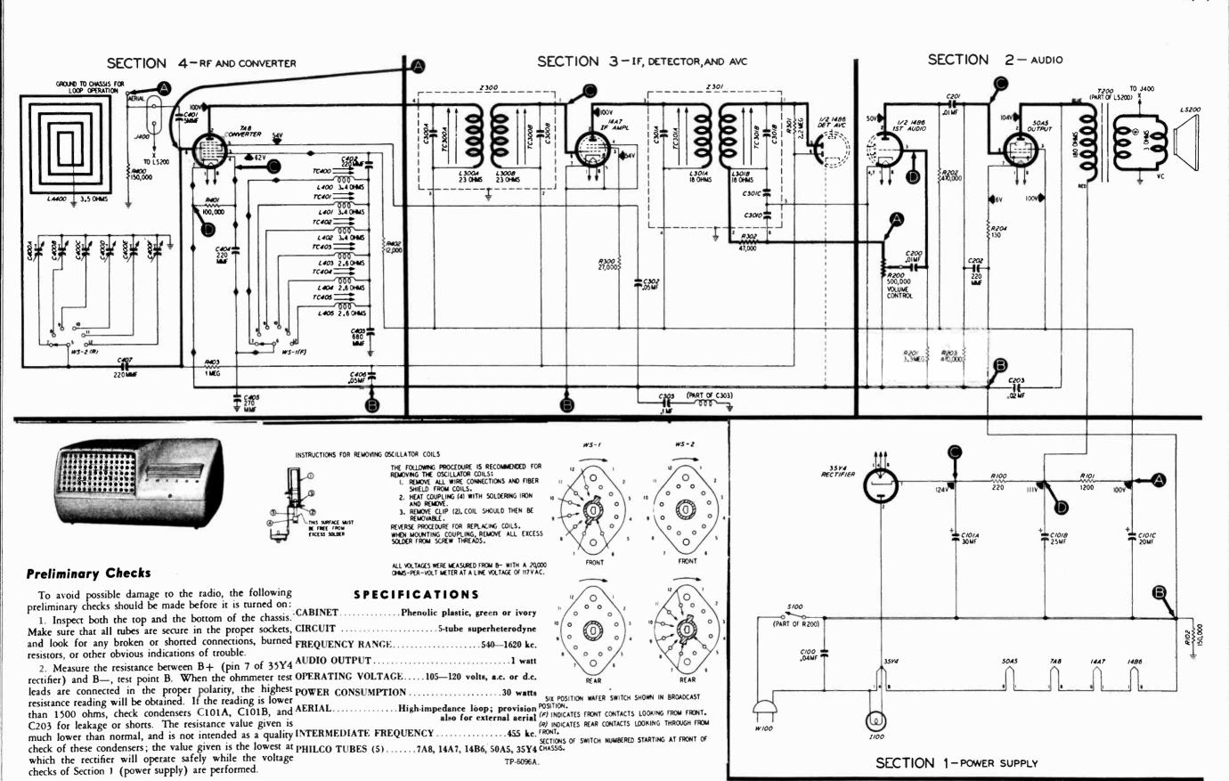
Figure 5. Philoo Radio Model 49-901, Sectionalized Schematic Diagram, Showing Test Points
