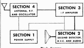
Block diagram (Heavy lines indicate signal path)
