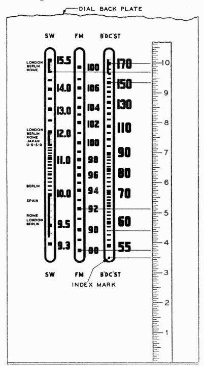
Figure 1. Calibration Measurements for Dial Backplate
