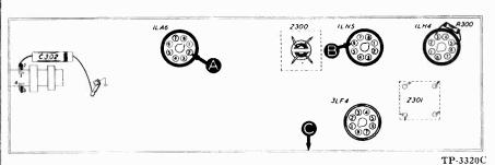
Figure 3. Bottom View, Showing Section 3 Test Points
