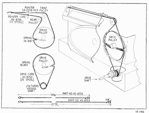
FIGURE 7. DRIVE-CORD INSTALLATION DETAILS
