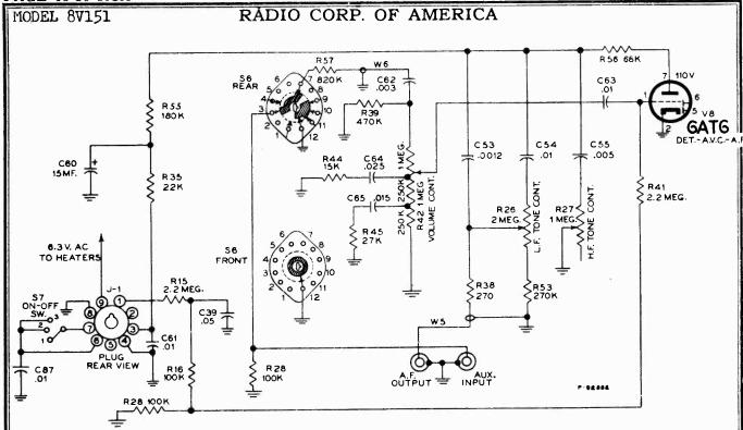
Simplified Schematic Diagram - Position. (AUX.).
