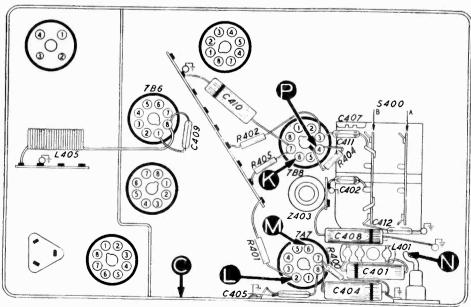
Bottom view, showing Section 4 test points.
