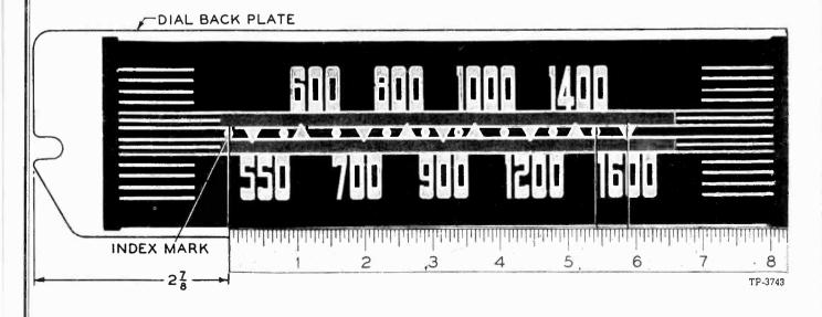
Figure 6. Calibration Measurements for Dial Backplate
