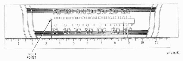
Figure 8. Composite Dial and Backplate, Calibration Details
