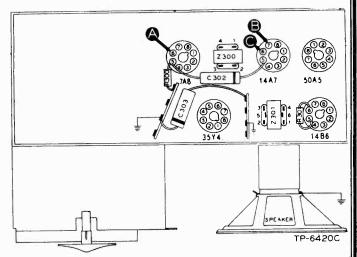
Figure 3. Bottom View, Showing Section 3 Test Points
