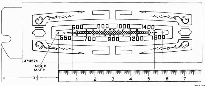
Figure 6. Calibration Measurements for Dial Backplate
