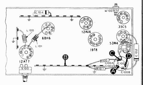
Figure 1. Bottom View. Showing Section 1 Test Points
