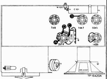
Figure 1. Bottom View, Showing Section 1 Test Points
