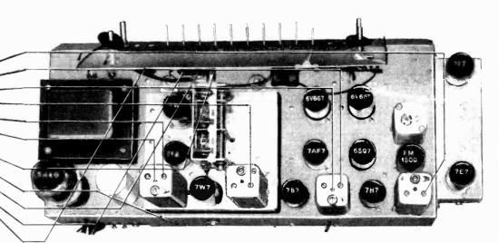
Figure 8. Top View, Showing AM Trimmer Locations
