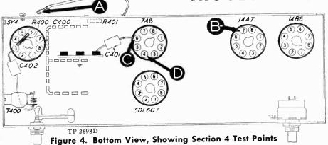
Make tests for this section by using an r-f signal generator with modulated output. Set frequency as noted in chart. Connect generator ground lead to B—; connect output lead through a .1-mf condenser to the test points indicated in the chart.
