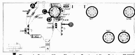
Figure 4. Bottom View, Showing Section 4 Test Points TP-3395D
