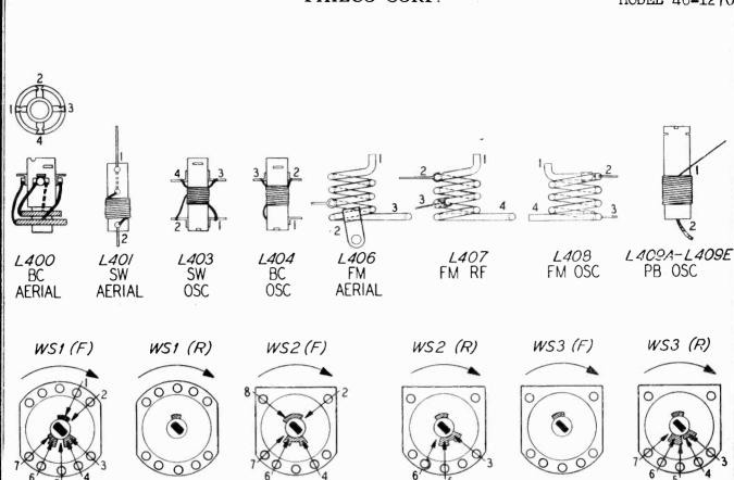
BAND-SWITCH SECTIONS SHOWN IN BROADCAST POSITION AS VIEWED FROM UNDER SIDE OF CHASSIS.
