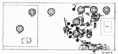
Figure 2. Bottom View, Showing Section 2 Test Points
