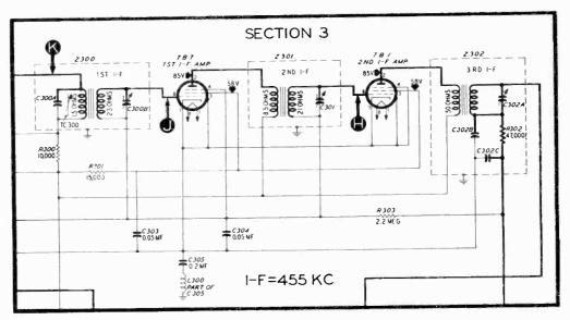
Figure 7. Section 3 schematic.
