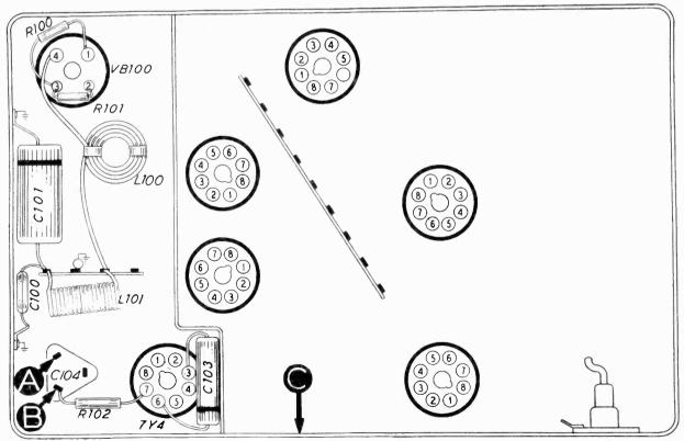
Bottom view, showing Section 1 test points.
