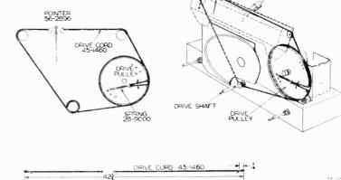
Figure 13. Drive cord installation details.
