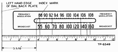
Figure 7. Dial-Backplate Calibration Measurements
