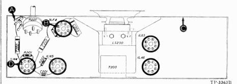
Figure 2. Bottom View, Showing Section 2 Test Points
