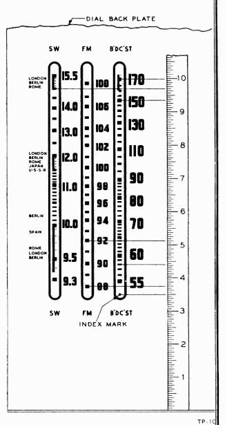
Figure 5. Calibration Measurements for Dial Backplate
