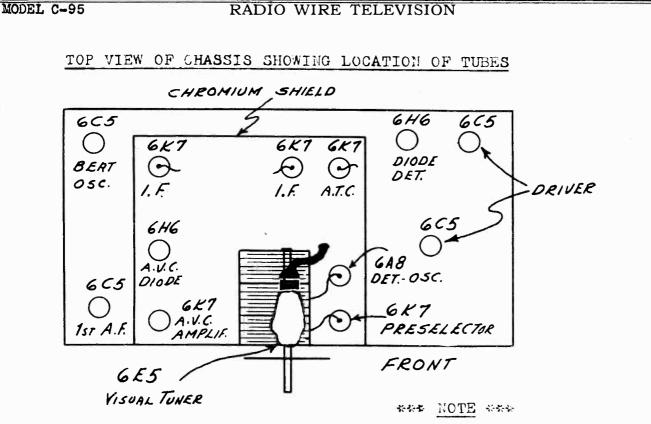
AUDIO OUTPUT AND RECTIFIER TUBES ARE IN POWER SUPPLY CHASSIS.
