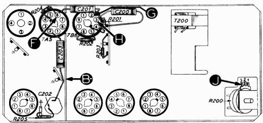
Bottom view, showing Section 2 test points.
