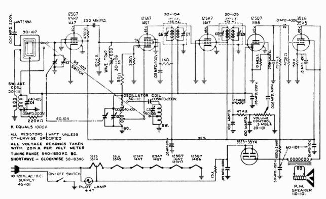
The Model 7162 is a 6 tube 2 band superheterodyne which will give reception over a wide range, including standard broadcast and foreign shortwave. The tuning range of the broadcast frequency is 540 to 1650 kilocycles, or 560 to 182 meters. The short wave frequency is 5.8 to 18.3 megacycles, or 16 to 49 meters, which includes the following: 16, 19, 25, 31, 39 and 49 meter bands.
