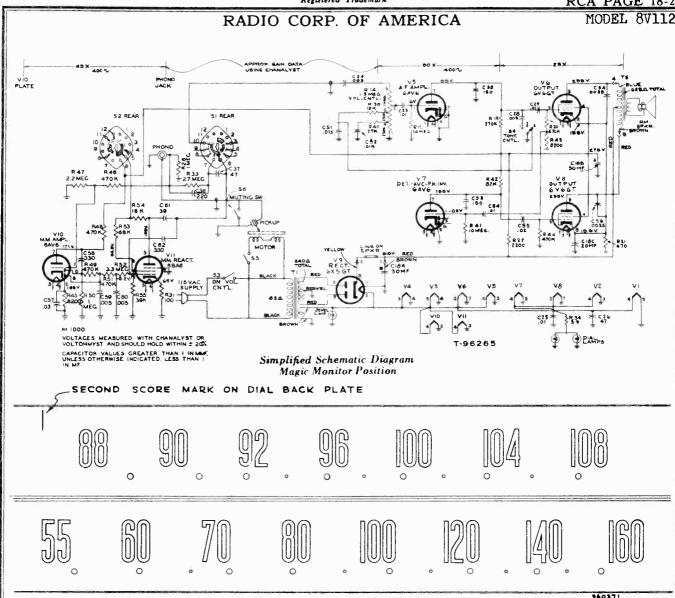
The dial scale drawing shown is a full size reproduction. It can be used as a reference in alignment procedure.
