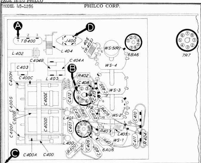
Figure 5. Bottom View, Showing Section 4 Test Points
