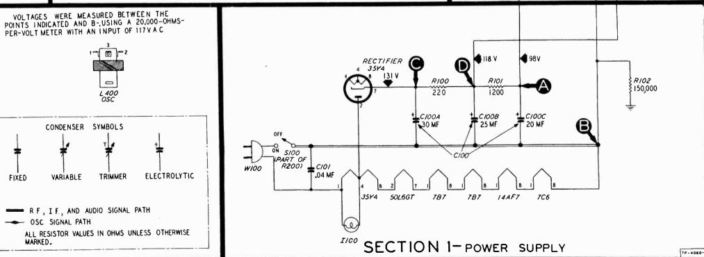
FIGURE 5. PHILCO RADIO, MODELS 49-900-E AND 49-900-I, SECTIONALIZED SCHEMATIC DIAGRAM, SHOWING TEST POINTS
