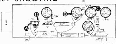
Figure 1. Bottom View, Showing Section 1 Test Points
