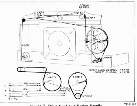
Figure 7. Drive-Cord Installation Details
