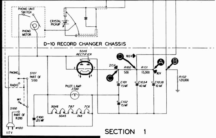
Figure S. Philcs Radio-Phonograph Models 48-1201 and 48-1260, Sectionalized Schematic Diagram, Showing Test Points
