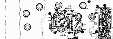
TP-4023B Bottom View, Showing Section 2 Test Points
