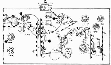
Figure 3. Bottom View, Showing Section 3 Test Points TP-6461
