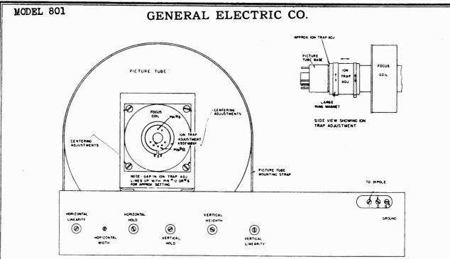
Fig. 17. Location of Installation Adjustment Controls
