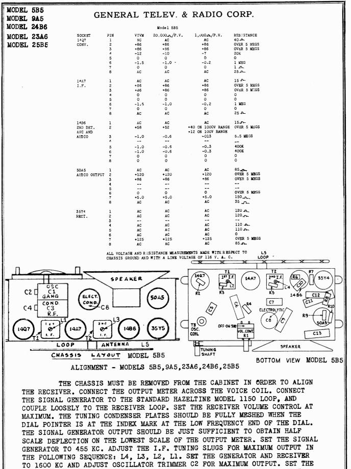
GENERATOR AND RECEIVER TO 1400 KC AND ADJUST R.F. TRIMMER C4 FOR MAX-
