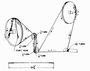
Fig. 15. Radio Tuning, Dial Drive Stringing
