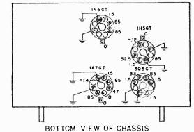
MEASUREMENTS TAKEN ON 20,000 OHMS PER VOLT METER. MEASURED FROM PIN TO CHASSIS. 1.5 V "A"-90 V "B" BATTERY PACK'. NO SIGNAL INPUT.
