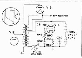
8. HIGH VOLTAGE SUPPLY (See Figure 6)-The high voltage is derived by making use of the inductive "kick" voltage pro-duced during retrace in the horizontal output transformer.
