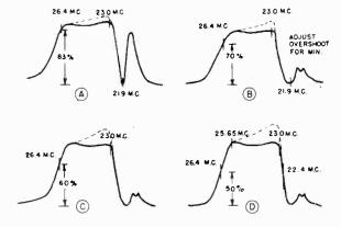
Fig. 9. Video I-F Alignment Curves
