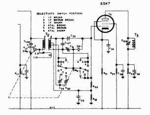
FIG. 2-CRYSTAL FILTER SCHEMATIC
