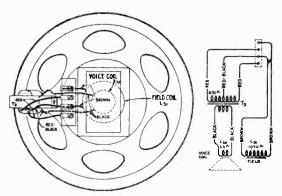
Figure 3—Console Loudspeaker Wiring
