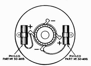
Fig. 9-Condensers Attached to Generator for Suppressing Interference
