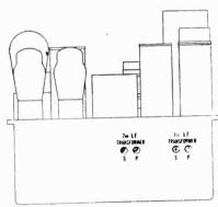
Figure C-I. F. Alignment Location
