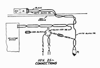
Figure G-100-115 Volt Connection of 25-60 Cycles Transformer
