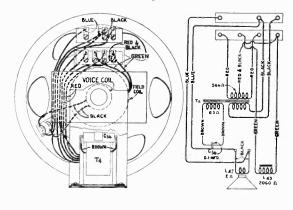
Figure 6—Loudspeaker Wiring
