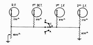
Figure 4—Sensitivity Control Switching Arrangement
