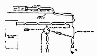
NOV. 25~ CONNECTIONS Figure G—100-115 Volt Connection of 25-60 Cycles Transformer
