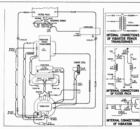
Figure 7—Vibrator Inverter-Rectifier Unit Wiring
