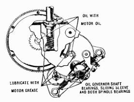
Figure A-Lubrication Diagram
