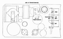
Figure C-Location of Line-up Capacitors
