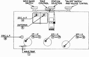
Fig. 1-Top View Showing Location of Compensating No. on Condensers.
