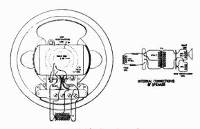
Figure 4—Table Loudspeaker Wiring
