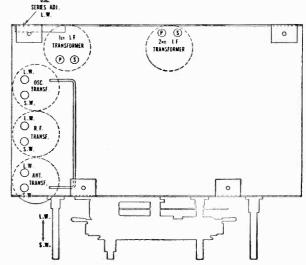
Figure D-Location of Line-Up Capacitors
