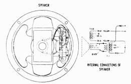
Figure D-Loudspeaker Wiring
