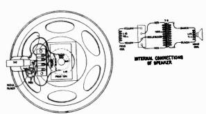
Figure 3—Loudspeaker Wiring
