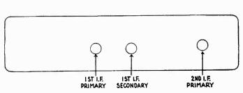
Fig. 3—Rear of Model 32 Chassis, showing location of I.F. Compensating Condensers. I.F. of Model 32 is 260 K. C.
