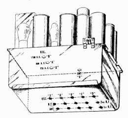
Figure F-Location of line-up capacitors
