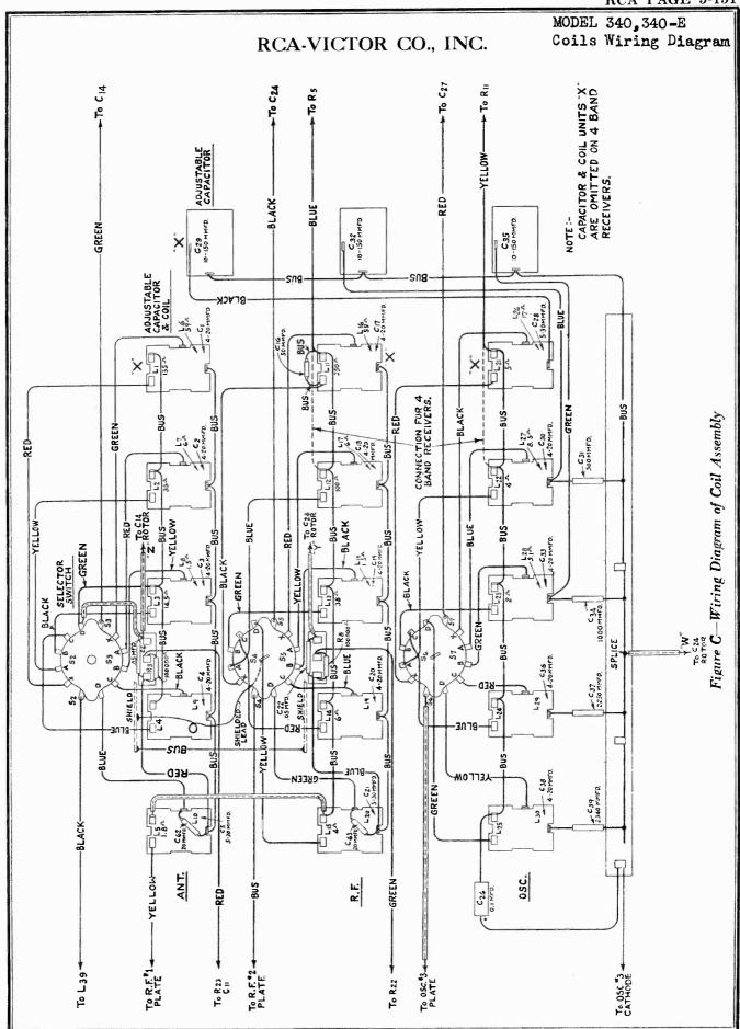
MODEL 340,340-E Assembly Wiring Voltage, Circuit Data
