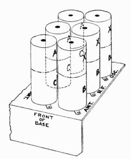
Figure 6-Location of Coils in Shields
