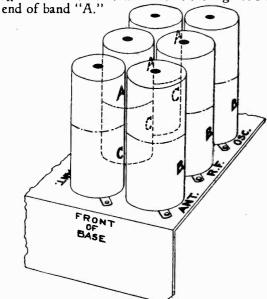
Figure 8-Location of Coils in Shields
