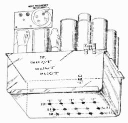
Figure E-Location of line-up capacitors.
