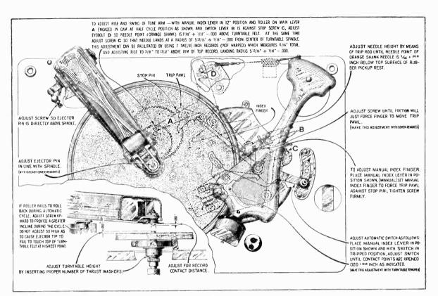
Figure E—Automatic Record Changer Adjustments
