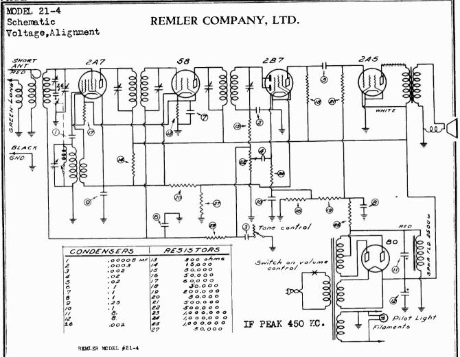
This radio receiver is of the superheterodyne type with automatic volume control.
