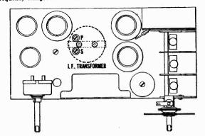
Figure C-Location of Line-Up Capacitors
