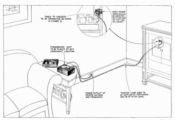
Figure 1—Typical Layout and Connections for Model R-93
