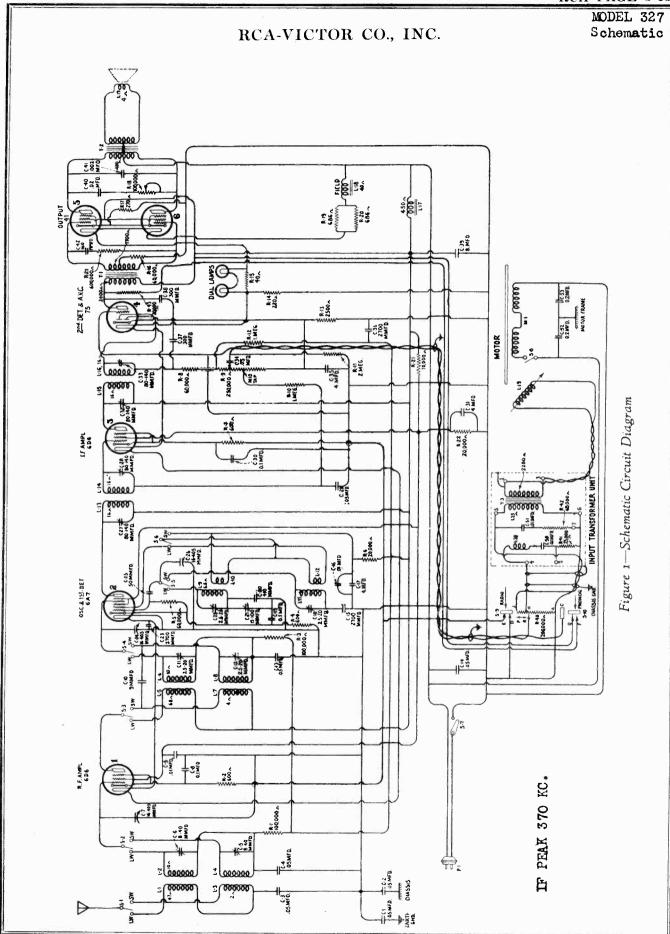
MODEL 327 Voltage Alignment Data Assembly Wiring
