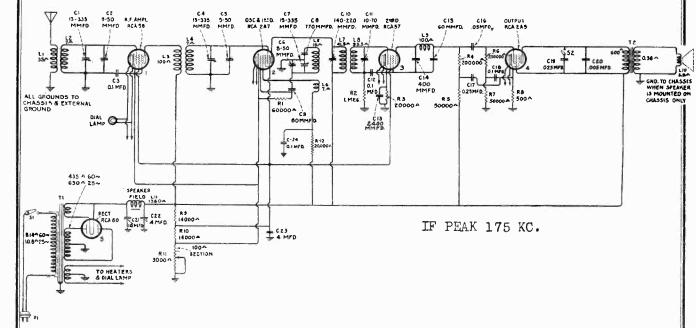
Figure 1-Schematic Circuit Diagram
