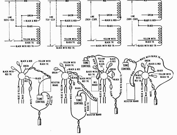
Figure H-Power Transformer Connections (50-60 cycles)
