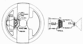
Figure 3—Loudspeaker Wiring
