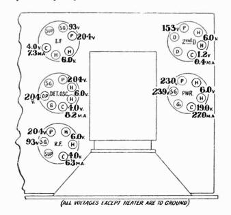
Figure 4-Voltages at Individual Socket Contacts
