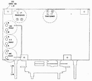
Figure E-Location of Line-Up Capacitors
