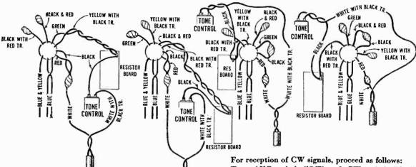
The power transformer of the 50-60 cycle receiver uses two tapped primary windings. By connecting them in parallel or in series, the receiver may be used either on 110 or 220 volt lines. Figure F shows the proper manner of making the various connections possible for this transformer.
