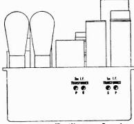
Figure 5-I. F. Alignment Location
