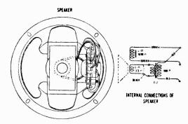
Figure C-Loudspeaker Wiring
