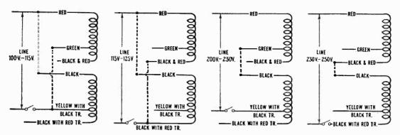
Figure F—Power Transformer Connections (50-60 cycles)
