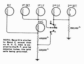
Figure 3—Switching Arrangement of Automatic Volume Control Systems
