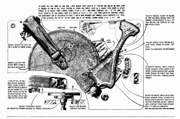
Figure 12—Automatic Record Changer Adjustments
