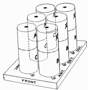
Figure 8-Location of Various Coils in Shields
