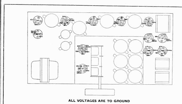
Figure 13—Radiotron Socket Voltages
