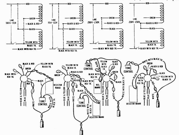
Figure H—Power Transformer Connections (50-60 cycles)
