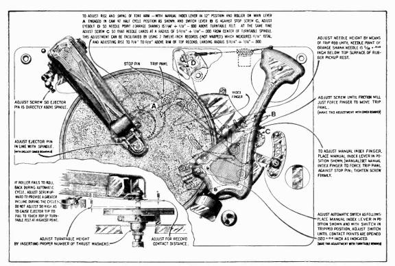
Figure H-Antomatic Record Changer Adjustments
