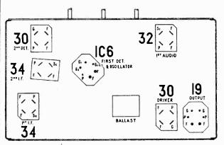
FIG. 3-Tube Socket Layout (View of Underside)
