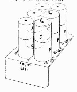
Figure 5-Location of Coils in Shields
