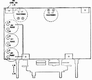
Figure D-Location of Line-Up Capacitors
