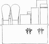
Figure 5-I. F. Alignment Location
