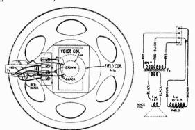
Figure 3—Loudspeaker Wiring
