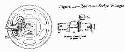
Figure 3—Loudspeaker Wiring
