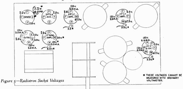
Volume Control at Maximum—No Signal—135 Volt "B" Battery—4.5 and 7.5-Volt Bias Batteries
