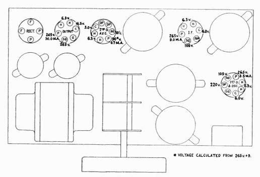
Figure 7—Radiotron Socket Voltages
