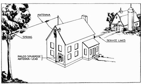
Fig. 8-Best Method of Antenna Installation for Model 32
