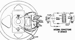
Figure 3—Loudspeaker Wiring
