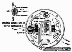
Figure 6-Loudspeaker Wiring
