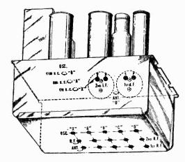
Figure F-Location of line-up capacitors.
