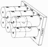
Figure 7—Location of Various Coils in Shields
