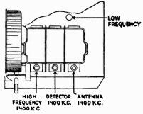
Fig. 4—Top View of Chassis Showing Compen-sating Condensers Mounted on Tuning Condenser, also Low Frequency Compensating Condenser.
