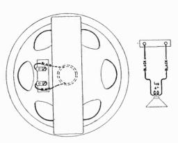
Figure 3—Loudspeaker Wiring
