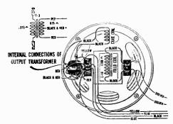
Figure 6-Loudspeaker Wiring
