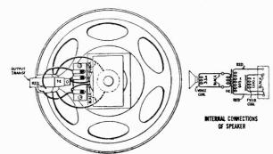
Figure C-Loudspeaker Wiring
