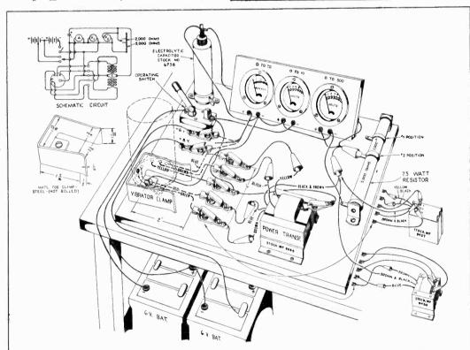
Typical Bench Set-Up for Testing Vibrators
