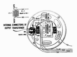
Figure D-Loudspeaker Wiring
