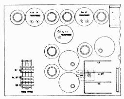
Figure D—Location of Line- Up Capacitors
