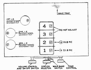
Fig. 5—Position of Compensating Condensers Reached from Above Chassis
