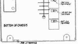
Fig. 2-Tube Arrangement & Location of Trimmers
