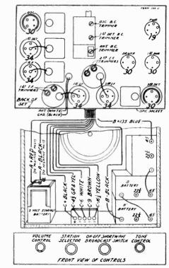
Fig. 2-Arrangement of Tubes, Batteries and Controls
