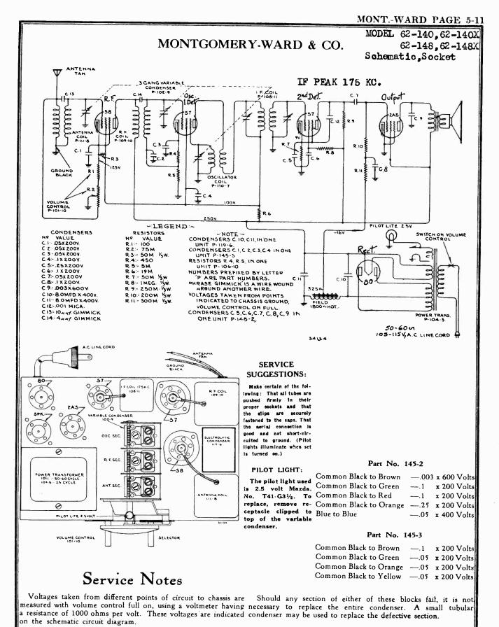
in good condition, until the defective unit is located. Part reproduction. numbers 145-2 and 145-3 are by pass condenser blocks and consist of the following condensers:
