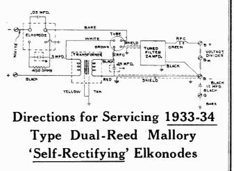
The 1933 Mallory Self-Rectifying Elkonode is a dual-reed converter which within itself sets up the essentially alternating current required, and likewise rectifies it to the form of direct current required for radio receiver plate supply. No rectifying tube is used with the 1933 Mallory Self-Rectifying Elkonode.
