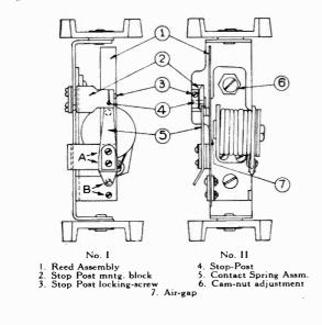
(1) is a side view showing the Elkonode with cover and rubber cushion removed. (2) is a front view with can and cushion removed. Numbered arrows clearly indicate the position of the Elkonode parts involved in installing new contact spring assemblies and new reed assemblies.
