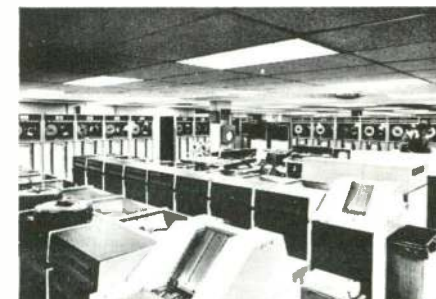
. . . Arbitron's two 3300 and twin 1700 Control Data computers. This is one of the largest on-premise computer operations in private industry.
