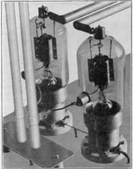
Figure 23. Parallel rod u.h.f. oscillator with HK-354C gammatrons in push-pull.
