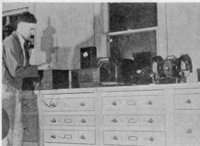
Figure 1. Most any corner having room for a bench and lots of drawer space can serve as the amateur's workshop. Drawers are preferable to shelves for storing radio parts since they will protect equipment from dust.
