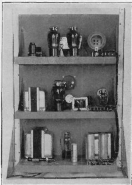
Figure 2. Back view of the 30-watt 160-meter phone transmitter. The r.f. unit, speech system and power supply are constructed on metal panels from which are supported metal chassis as illustrated. A hardwood rack can be used to support the panels if a suitable metal one cannot be obtained or if the required metal tools for construction of a metal rack are not available.
