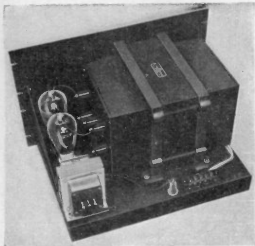
Figure 31. The heavy-duty high-voltage power transformer and the rectifiers are mounted on the bottom rack.
