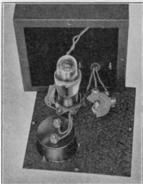
Figure 5. There are few components inside can housing the diode-type field-strength meter. A single "little six" dry cell is strapped inside the cabinet and supplies 1\frac{1}{2} volts to the filament of the type-30 tube, used as a diode rectifier.
