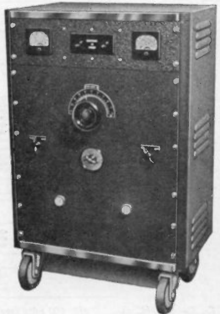
Figure 4. This de luxe 400-watt u.h.f. diathermy machine incorporates many safety features and worthwhile refinements. It uses two HF-200's in a push-pull Armstrong circuit.
