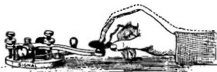
Correct position for arm and wrist, showing how third and forefinger and thumb are placed on key knob.
