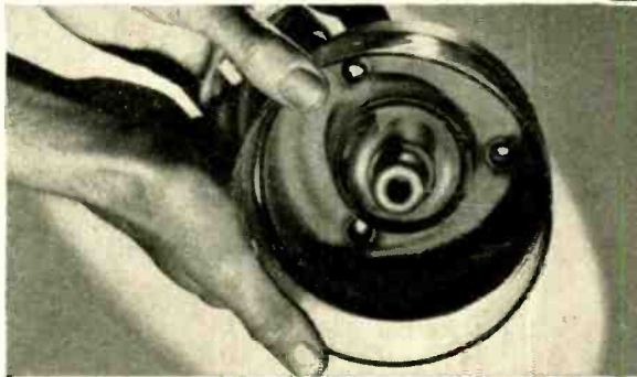
There are four complicated glass to metal seals in this vacuum tube part
