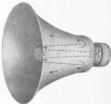
Left: MARINE HORN Speaker, approved by the U. S. Coast Guard. Several sizes available, Stormproofed, of the re-entrant type, suitable for indoor or outdoor use—may be used as both speaker and microphone. Right: RE-ENTRANT TRUMPET; available in 3½', 4½' and 6' sizes. Compact. Delivers highly concentrated sound with great efficiency over long distances.
